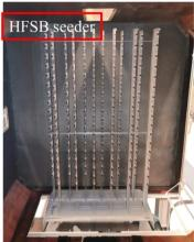
Figure 5.1: Experimental set up: Robotic PIV measuring (left), HFSB seeder inside the settling chamber of W-tunnel (right).
