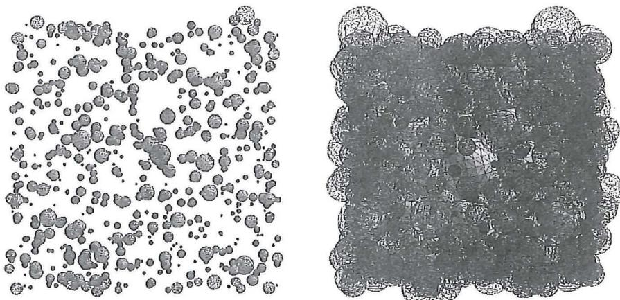
Figure 3. Spherical particles dynamically compacted from loose (left) into dense random state (right) by the DEM system HADES
