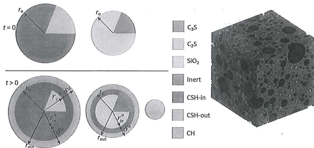
Figure 4. Particle models of cement, pozzolanic admixture and hydration product (at the left) and visualized microstructure (at the right)
