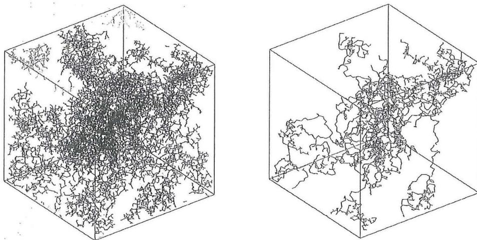
Figure 7. Pore delineation in 100μm cubes for gap-graded blended-PC. All capillary pores are shown (left) as well as the continuous trunks only (right). Visually similar results were obtained for plain PC
