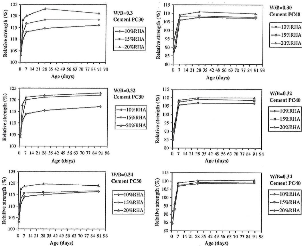
Figure 1. Relative compressive strength values of gap-graded aggregate RHA-blended concrete
