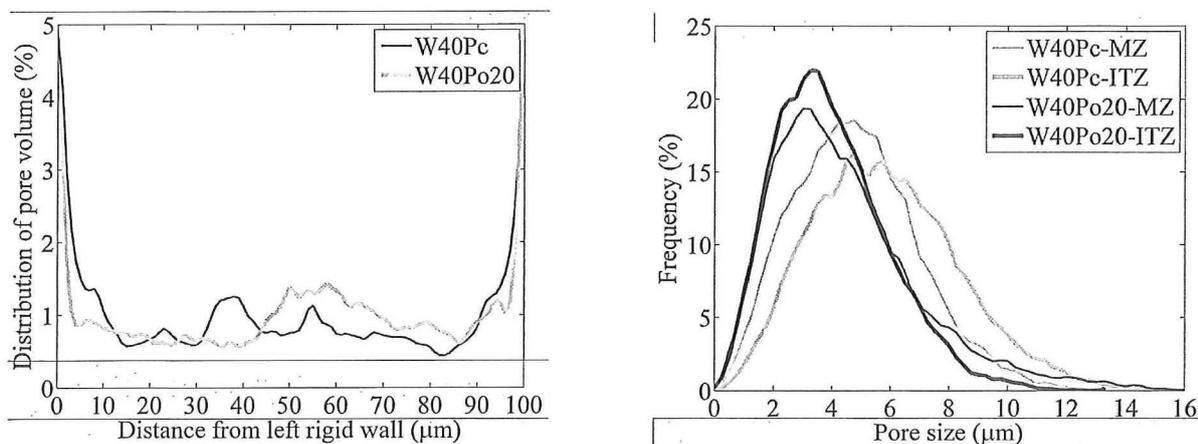
Figure 8. Effect of blending on ITZ extension (left) and on volume-based pore size distribution in and outside the ITZ zone (= Middle Zone).
