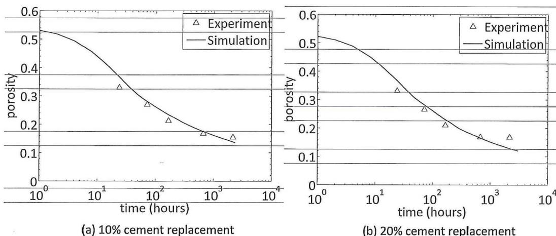
Figure 5. Porosity of the RHA-blended PC samples (the experimental results are derived from testing of Nguyen (2011b) on RHA-blended PC samples with  $w/b = 0.4$  and 10-20% replacement).
