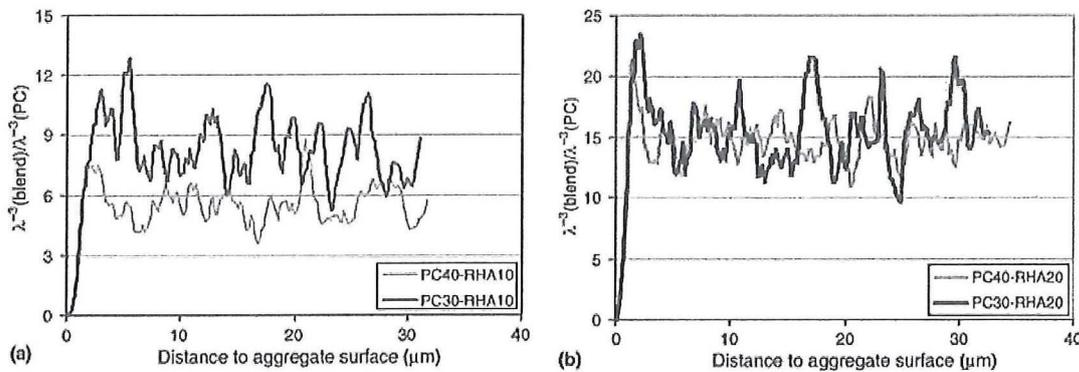
Figure 2. RHA blending reveals increased density in virtual concrete when gap-graded with the coarser PC.  $\lambda^{-3}$  is supposedly proportional to global van der Waals bond, whereby  $\lambda$  is the mean free spacing.
