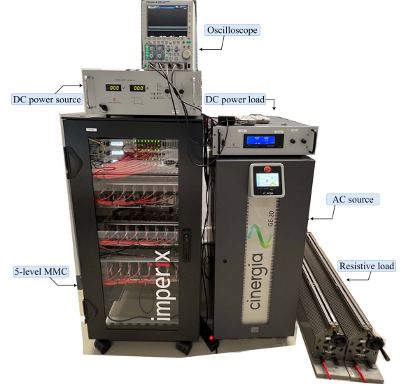
Fig. 15. Experimental setup with MMC prototype.
