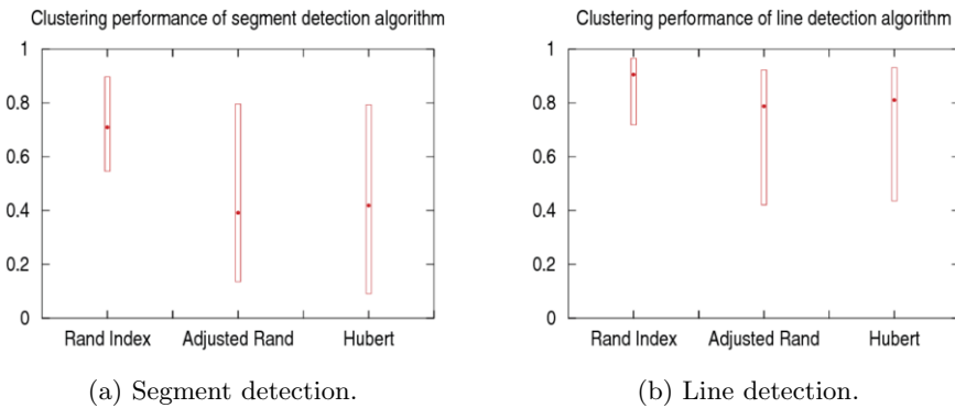
Figure 5. Segment detection performs much worse than line detection across all three clustering performance indicators. Perfect clustering is indicated by 1.0 for Rand Index, Adjusted Rand Index, and Hubert.
