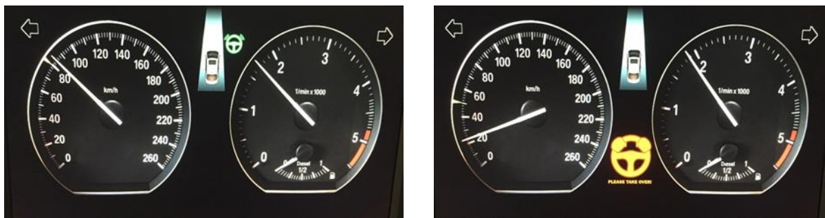
Figure 3. Photos of the instrument cluster with automation status. Left: automation available, corresponding to Figure 2b; Right: take-over request, corresponding to Figure 2e.
