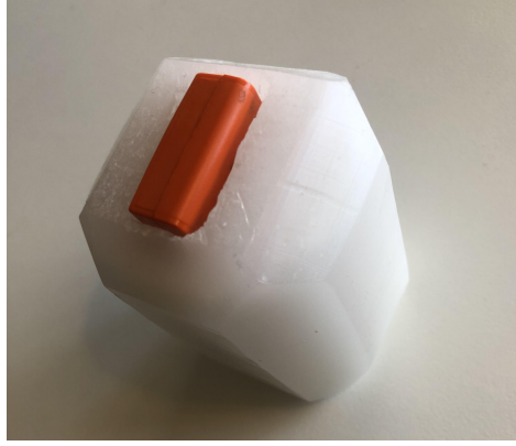
Figure 3-2: An orientation prism with 18 faces in which the Xsens MTw can be placed to obtain stationary acceleration data for these 18 different orientations.
