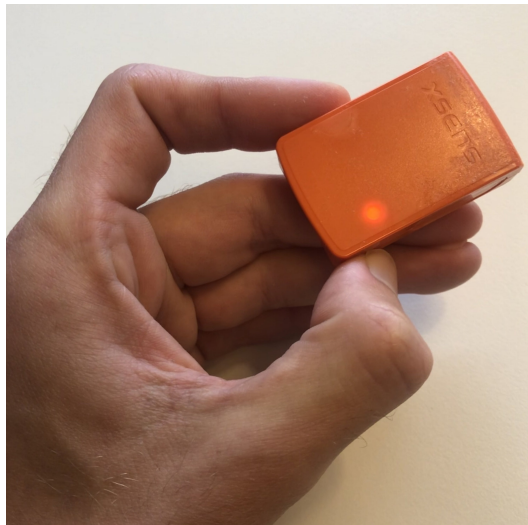
Figure 1-1: The Xsens MTw Awinda wireless IMU sensor [11].
