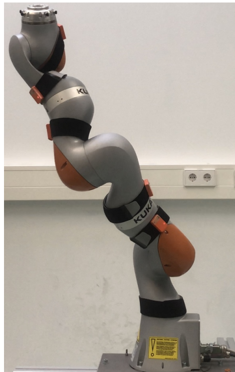
Figure 5-1: The KUKA LBR iiwa 7 R800 robot with the six Xsens MTw Awinda IMUs.
