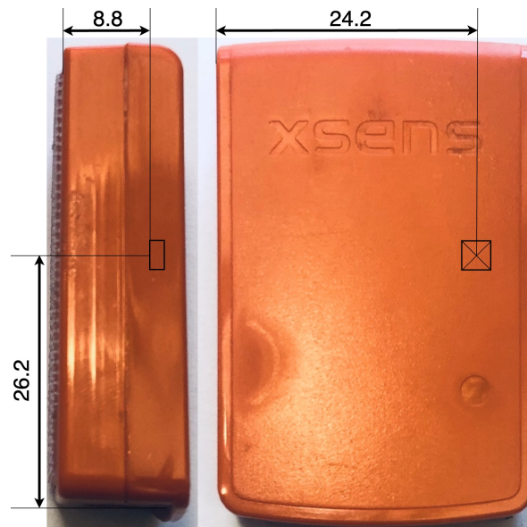
Figure F-2: Schematics of the accelerometer position in the Xsens MTw Awinda IMU. Distances are shown in [mm]. Figure adapted from [48].
