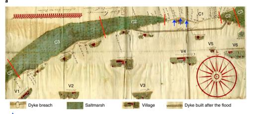
Each blue arrow points to a mega breach ('met meyvelt gelyck': the dyke section had completely disappeared)
