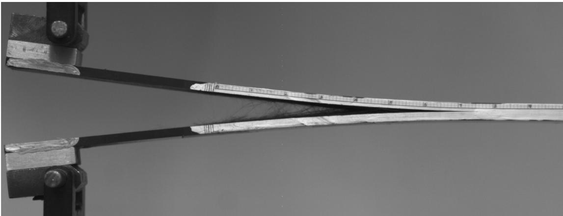
**Figure 6.4:** Side view of a specimen tested by Yao showing signs of fibre bridging
