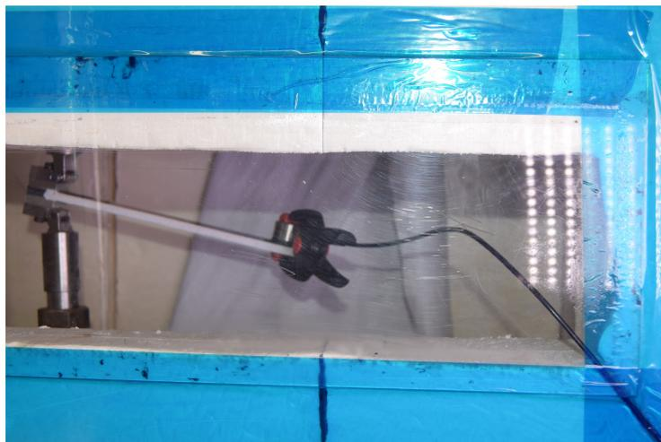
**Figure 4.4:** detail from experimental setup for DCB testing at different temperatures depicting the test specimen attached to the fatigue machine
