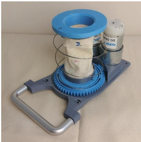
Figure 5: Picture of the Twisting-Tube gripper prototype.
