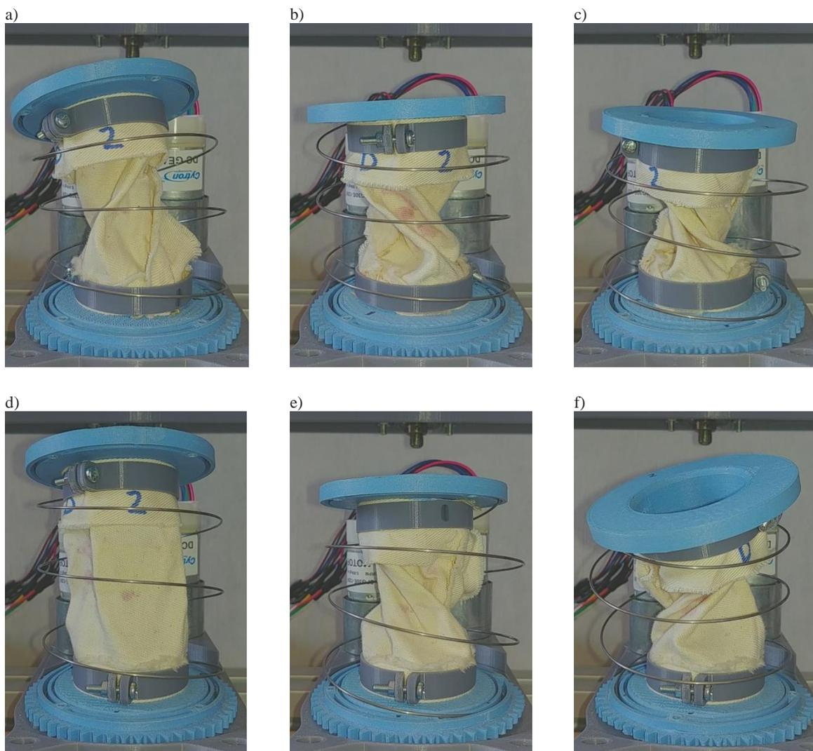
Figure 9: Stills of gripping procedure without an object inside. a,b) Tube rotates bottom ring 110 degrees clockwise and counter clockwise to aid an object in entering the tube. c) Tube twists close. d) Tube returns to initial open position. e,f) Tube rotates top ring 110 degrees clockwise and counter clockwise to aid an object leaving the tube.
