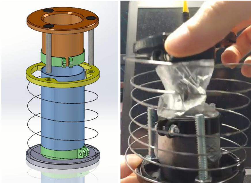
Figure 19: On the left is a screenshot of the CAD design of the first prototype Twisting-Tube gripper, with in green split rings which clamp the blue tube in place and in yellow an adjustable stage to tension the spring. On the right is a still of a video in which the gripper gets tightened using a plastic, see-through tube.
