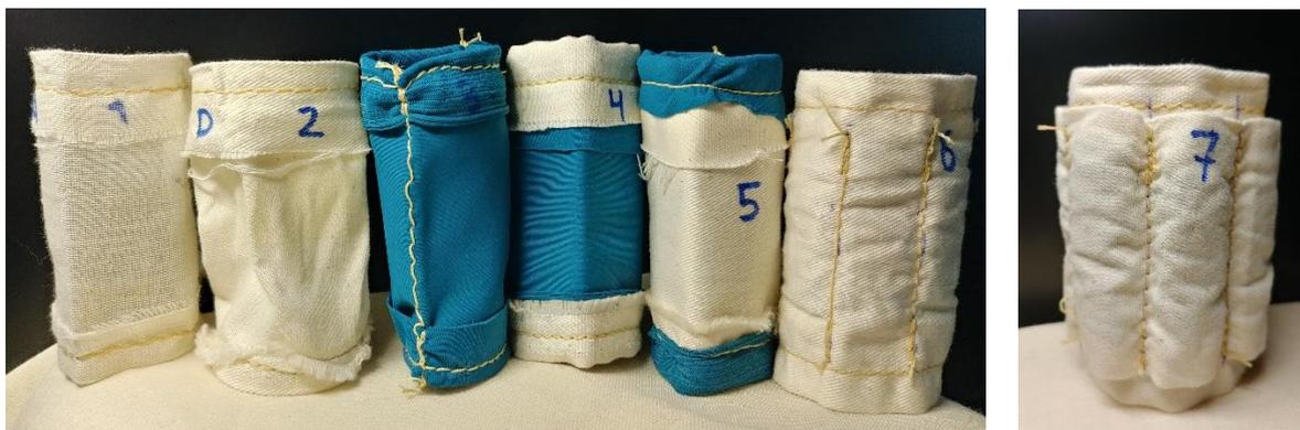
Figure 7: The seven tubes used in testing the blackberries. From left to right, the presentation order is the same as in Table 2. The cheesecloth is white, and the spandex is blue. Tube 7 seen in the picture on the right is the same tube as number six seen on the left but turned inside out.
