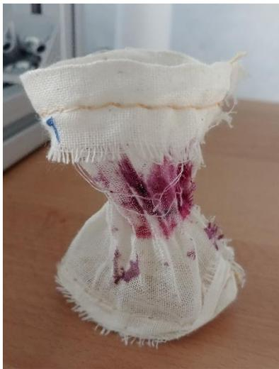
Figure 18: The thin cheesecloth tube after testing, noticeable are the many stains in the middle of the tube due to leaking drupelets. This type of tube stayed wrinkled during and after testing, probably due to the dried up blackberry fluid and the thinness of the material.
