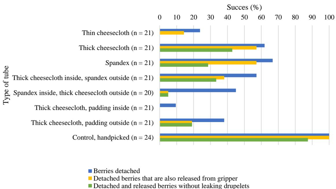
Figure 16: The number of berries after each of the performance checks: detachment, releasement and no leaking drupelets.
