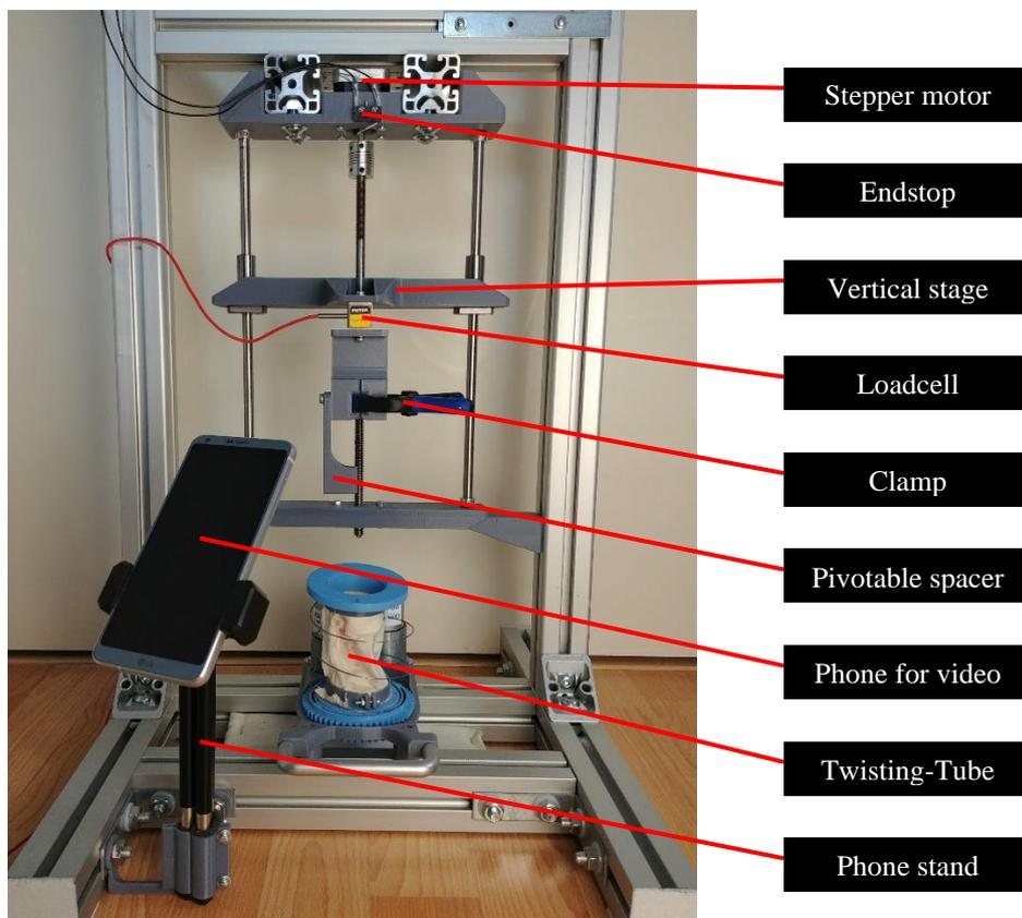
Figure 8: Measurement setup. A stepper motor powers a vertical stage that connects to a clamp for holding the blackberries via a loadcell. The phone shoots a video of the closing procedure of the Twisting-Tube gripper at the bottom.
