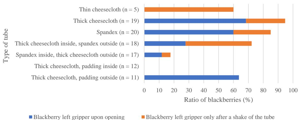
Figure 13: Ratio of tested upon blackberries that left the gripper successfully after being detached from the pedicel during opening or the subsequent shake of the tube.
