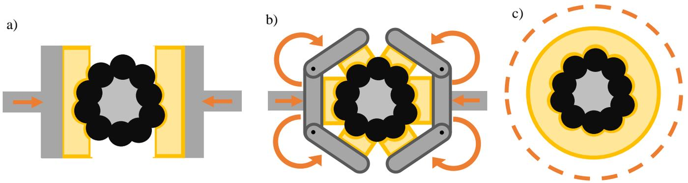
Figure 2: Top view of three different approaches to the soft berry in the middle. a) shows two hard surfaces (grey) that approach the berry with a deformable layer (yellow). b) shows six hard surfaces (grey) that pivot and approach the berry from more sides with deformable layers (yellow). c) shows only deformable components (yellow) which interact with the berry by decreasing in diameter and closing in around all sides of the berry.
