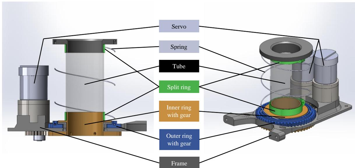
Figure 4: CAD drawings made in SOLIDWORKS, on the left a cross section of the model and on the right an 3D view. Fasteners are removed and the tube is made partly transparent in this drawing to better see the mechanism.
