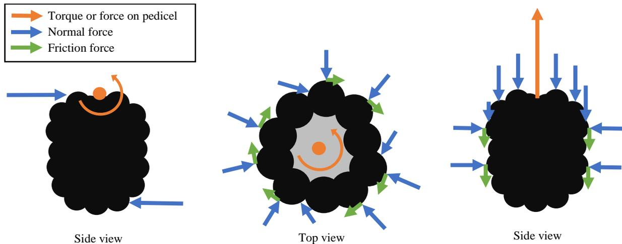
Figure 1: Free body diagrams of a blackberry during pedicel detachment movements. On the left a bending movement that imposes a torque around the pedicel (orange), in the middle a top view with a torque (orange) around the major axis of the berry, and on the right a pull force on the pedicel in orange. Exemplary normal forces are shown in blue and exemplary friction forces in green. Depending on the contact points the gripper is able to make, these forces can differ in size, and where they act.
