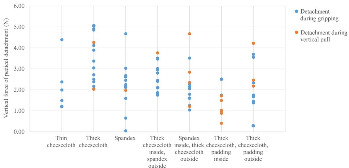
Figure 14: Vertical force necessary for successful detachment of the blackberry during gripping (blue) and during the subsequent vertical pull (orange), each dot represents a test on a single blackberry.
