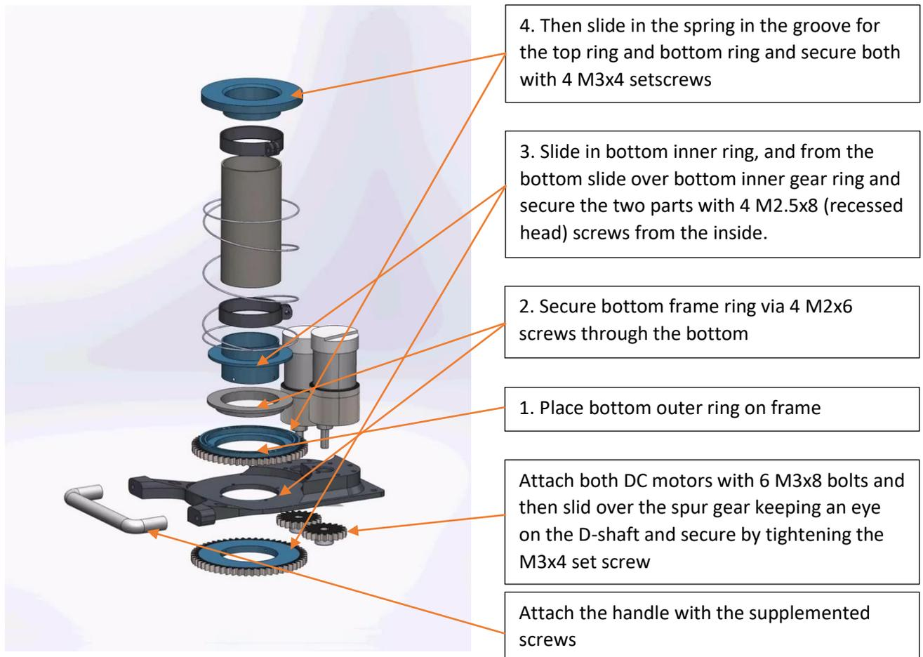
Figure 22: Exploded view of the Twisting-Tube gripper. On the right, the correct numbered order can be seen to assemble the gripper. The handle, motors and cloth can be installed and removed without needing to disassemble the entire gripper. Replacing the cloth is made especially easy by untightening the split rings that hold it in place at either end, this allowed for relatively quick replacement during testing of the gripper.
