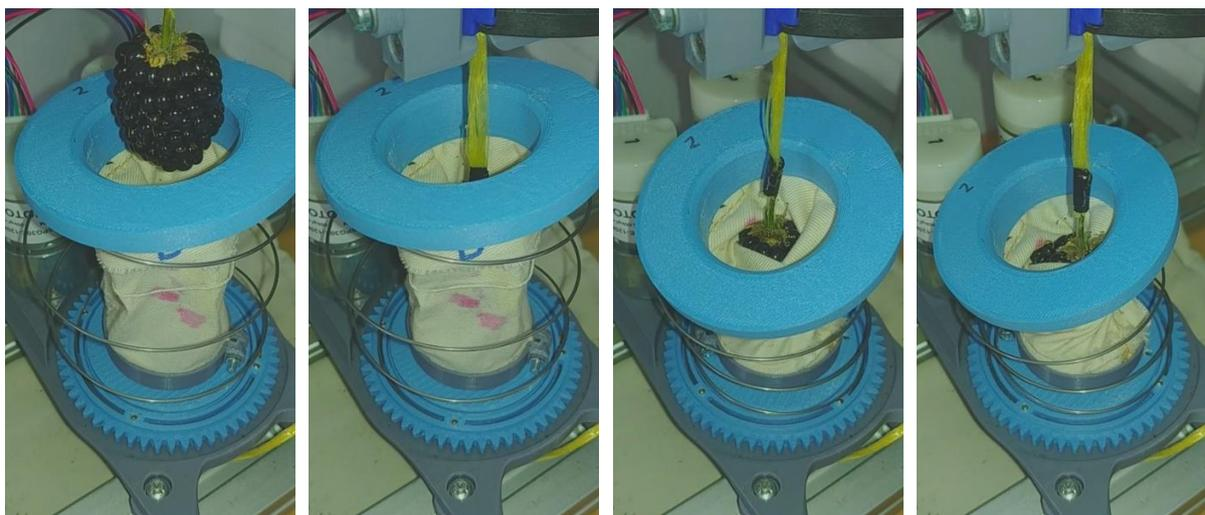
Figure 12: From left to right, pictures of a single pedicel removal procedure can be seen for the Twisting-Tube gripper equipped with thick cheesecloth. The blackberry enters, the tube twists and tightens around the berry, and in the final picture the pedicel is detached from the berry.
