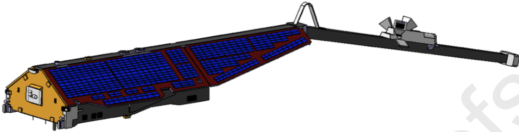
Figure 4: Rendering of the March et al. (2019a) high-fidelity 3D outer surface geometry model for Swarm.
