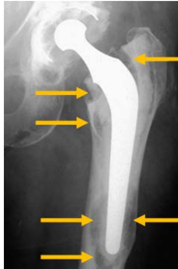
Figure 2.2: Aseptic loosening after total hip arthroplasty, with extensive osteolysis around the femoral component (shown with the arrows) and mechanical failure of the prosthesis, resulting in aseptic loosening [Wilkinson 2011].
