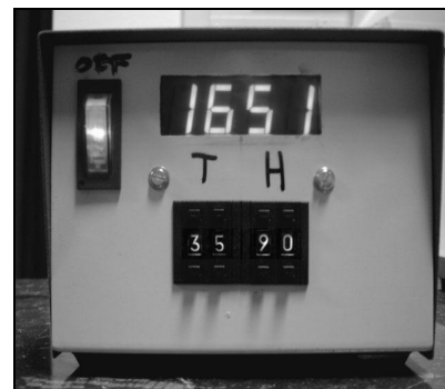
Figure 5: Control box for the required temperature and humidity
