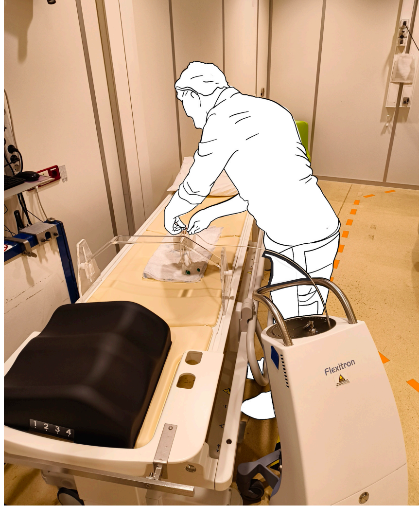
Figure 98: Testing the possibility of the radioactive source passing through the curves of the catheters with the flexitron afterloader.
