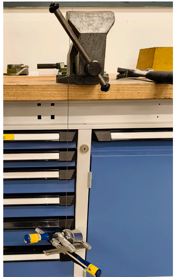
Figure 50: The pre-tensing setup for Nitinol testing
