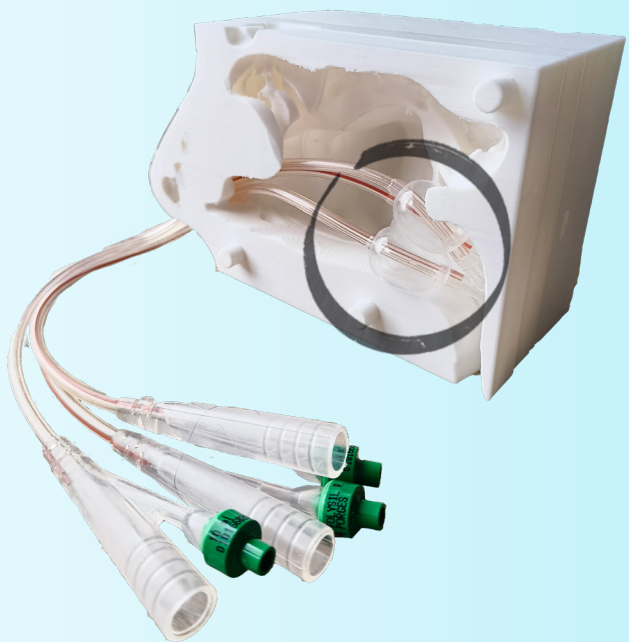
Figure 83: Testing the freedom of the original PORGES-14 applicators inside of the 1.5x scaled phantom
