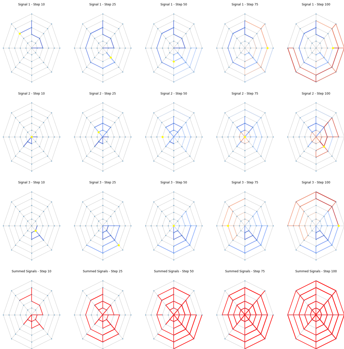
Figure 4.3: The following image presents a series of snapshots showing signal propagation and collisions over time in a spider web lattice. The top three rows illustrate individual signals moving through the structure, while the bottom row shows the cumulative effect of multiple signals interacting. The intensity of the red lines in the final frames highlights regions with higher collision frequencies and coverage of the web.
