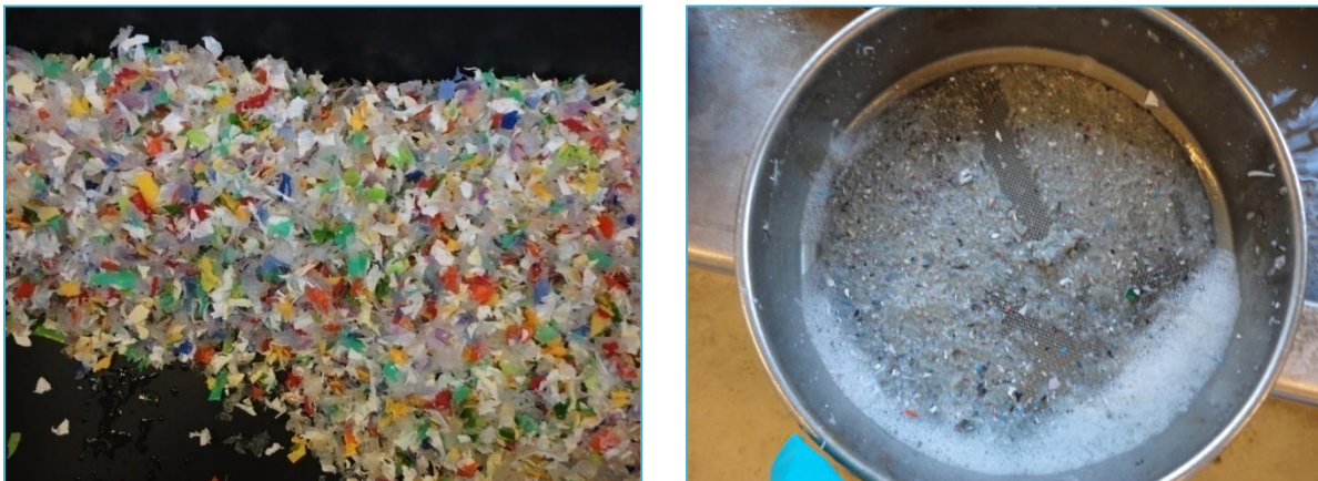
Figure 49: Second step of cleaning: Cleaned PP blow mold flakes (left), filtered impurities (right)
