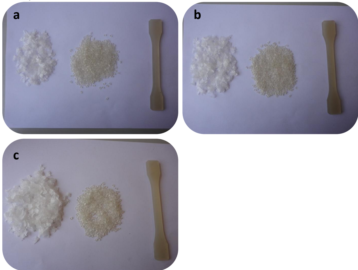
Figure 53: optical properties of flakes, granules and injection molded sample of PP thermoformed and blow mold grades from specific products: a) Bami boxes; b) vegetable boxes; c) Persil bottles.
