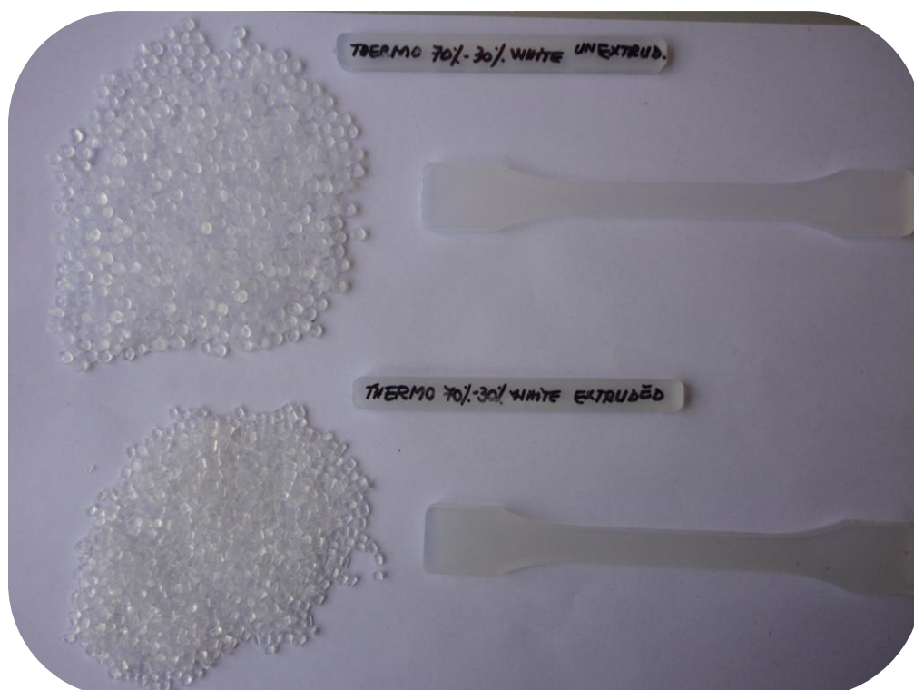
Figure 55: optical properties of flakes, granules and injection molded sample of PP virgin injection mold grade before and after extrusion
