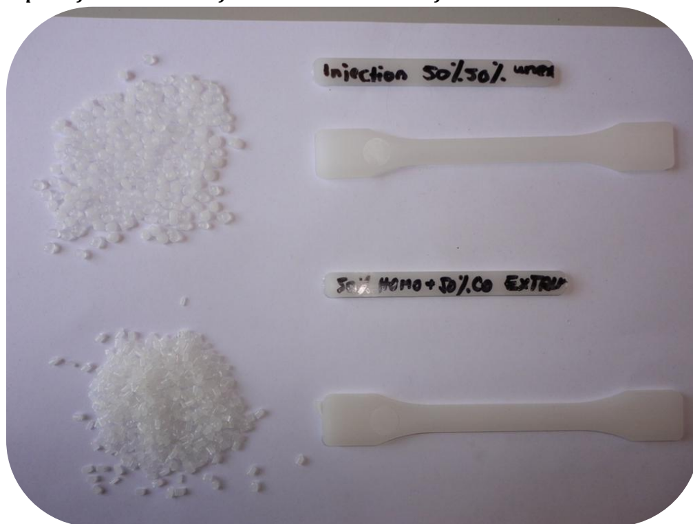
Figure 54: optical properties of flakes, granules and injection molded sample of PP virgin injection mold grade before and after extrusion
