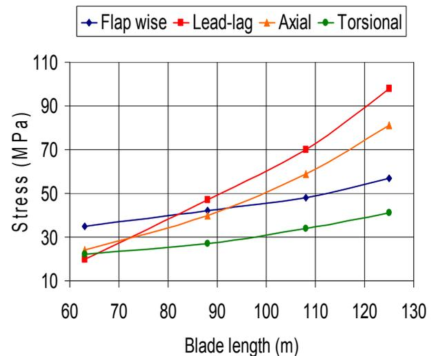
Figure 7: Change of stresses with size
