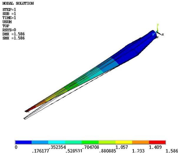
Figure 1: Deformation plot of the blade, colors indicate the total displacements of the blade
