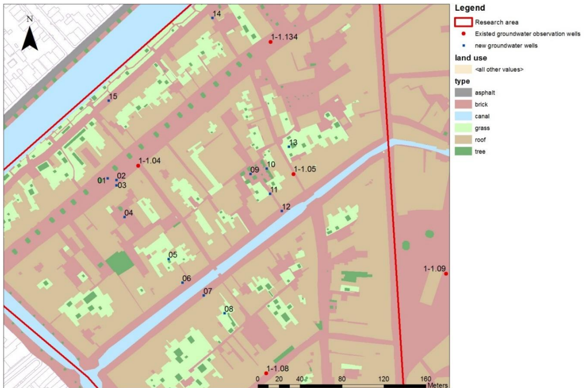
Figure 23 Locations of all the wells in the new groundwater observation network
