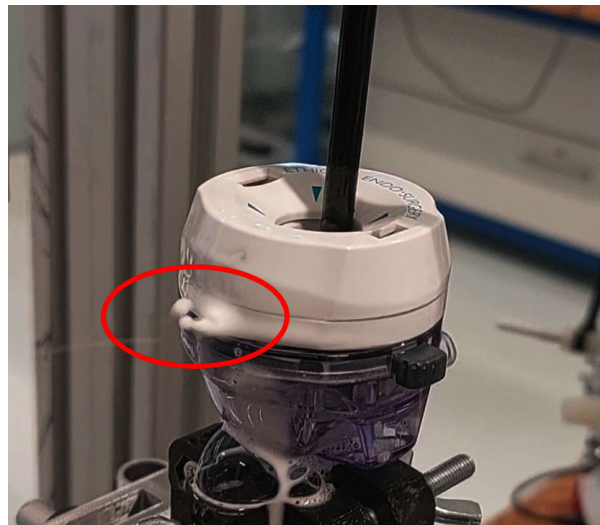
Fig. 14: Soap bubbles showing leakage between head and body of trocar 17
