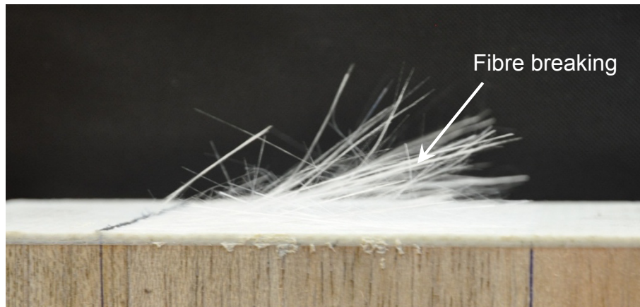
Fig. 5.33. Combination of fibre breaking and interfacial failure between adhesive layer and FRP laminates (T-SB-03)
