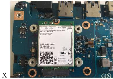
Fig. 1. INTEL's WiGig sink chipset W13100.
