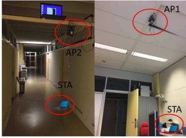
Fig. 15. Experimental scenario for handoff triggered by corner effects.
