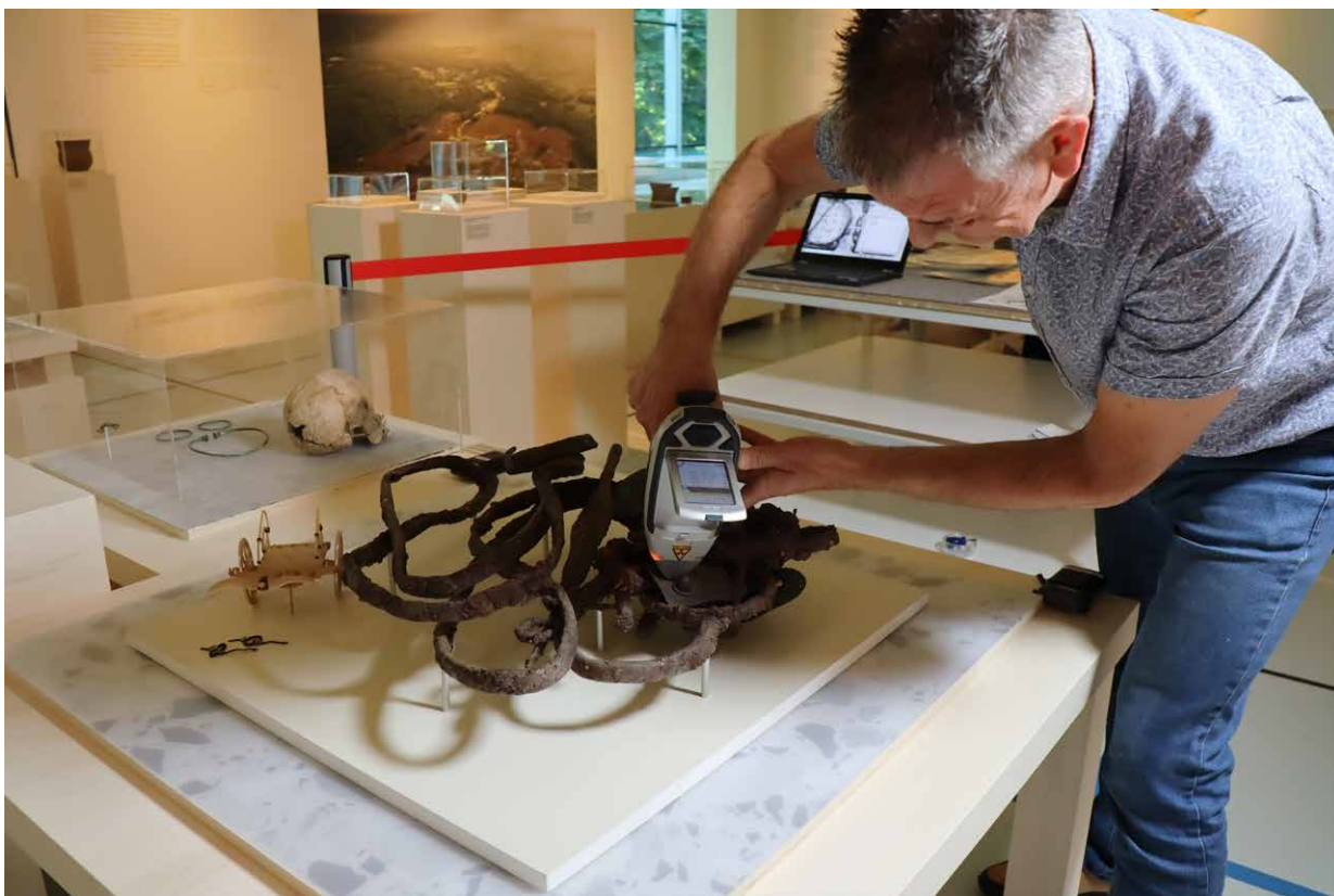
Fig. 10.1. The use of the Niton XL3t GOLDD+ XRF analyser on the remains from the chariot grave of Nijmegen-Traianusplein (RCE).
