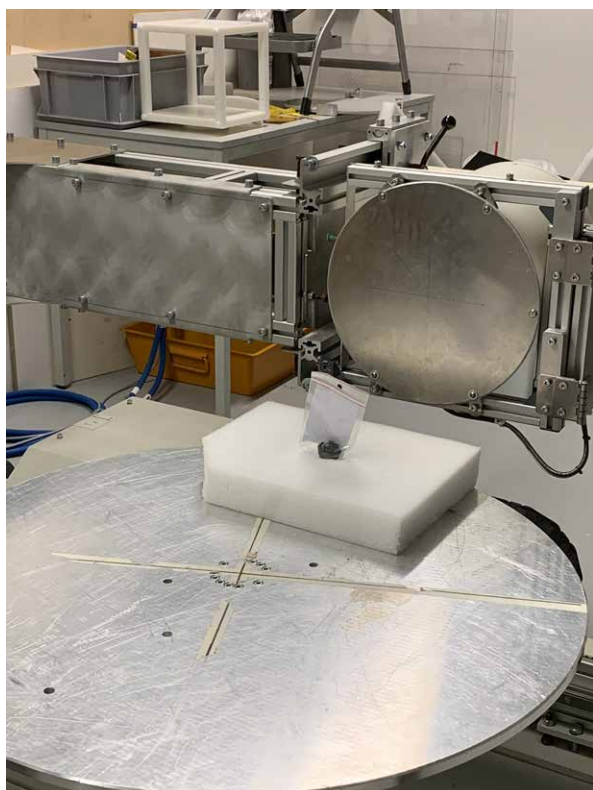
Fig. 10.8. Hollow spherical ball Heumen-17 in the X-ray setup at the Cultural Heritage Laboratory in Amsterdam (left), and the 120kV, 4 mA-image (right) (RCE).
