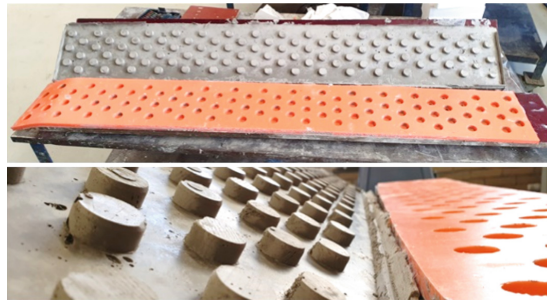
Fig. 2. Shearkeys in profiled SHCC laminates.
