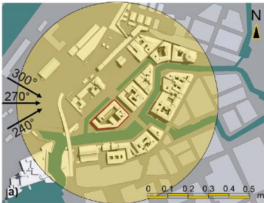
Geometry (Digital model) and different wind angles ( Ricci et al., 2017 )
