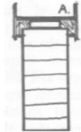
Figure 15: Good metal flashing with air space, drips, and polyethylene sheet (Schein, 1968)
