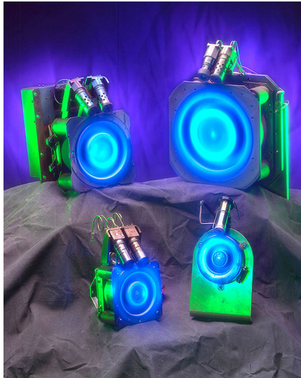
Figure 3.2: Stationary Plasma Thruster family. The SPT-100 is at the top left corner ( NASA/Glenn Research Center 1997 ).
