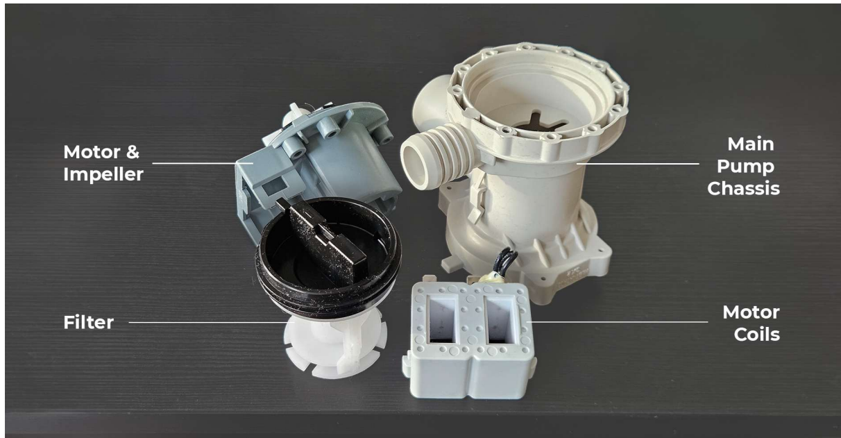
Figure 4: Disassembly of the reference pump and its four main components (photograph taken by author).
