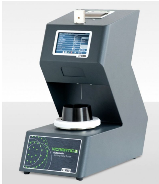
Figure 4.5: The automatic Vicat apparatus that is used in this study. (Automatic Vicat Apparatus, n.d.).
