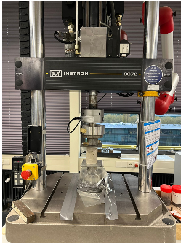
Figure 4.13: Test setup for the uniaxial unconfined compressive strength, with the Instron machine. Cylindrical samples have a diameter of 53 mm and a height of 95 mm.
