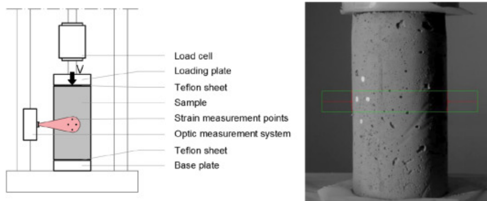
Figure 4.12: Schematic of uniaxial unconfined compression test (left) and photograph of a sample (right). The white dots are strain measurements points. ( Wolfs et al., 2018 ).
