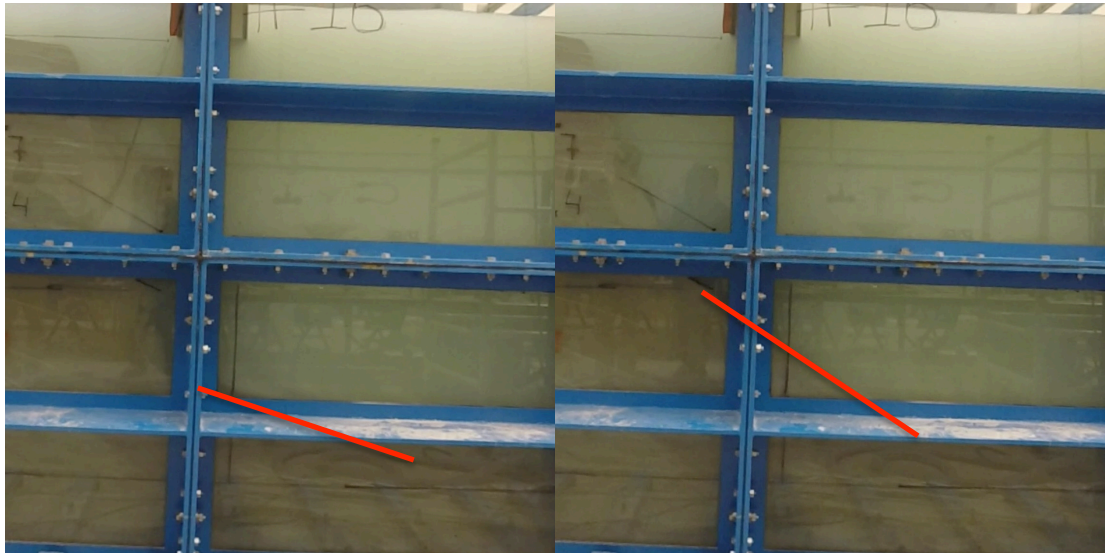
Figure 5- 29: A large sliding wedge, which result into a steep angle at the toe.
