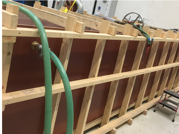
Figure 3- 4: The sedimentation tank
