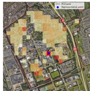
Figure 4.4: Example of selecting the representative point for postcode 2628 (Delft)
