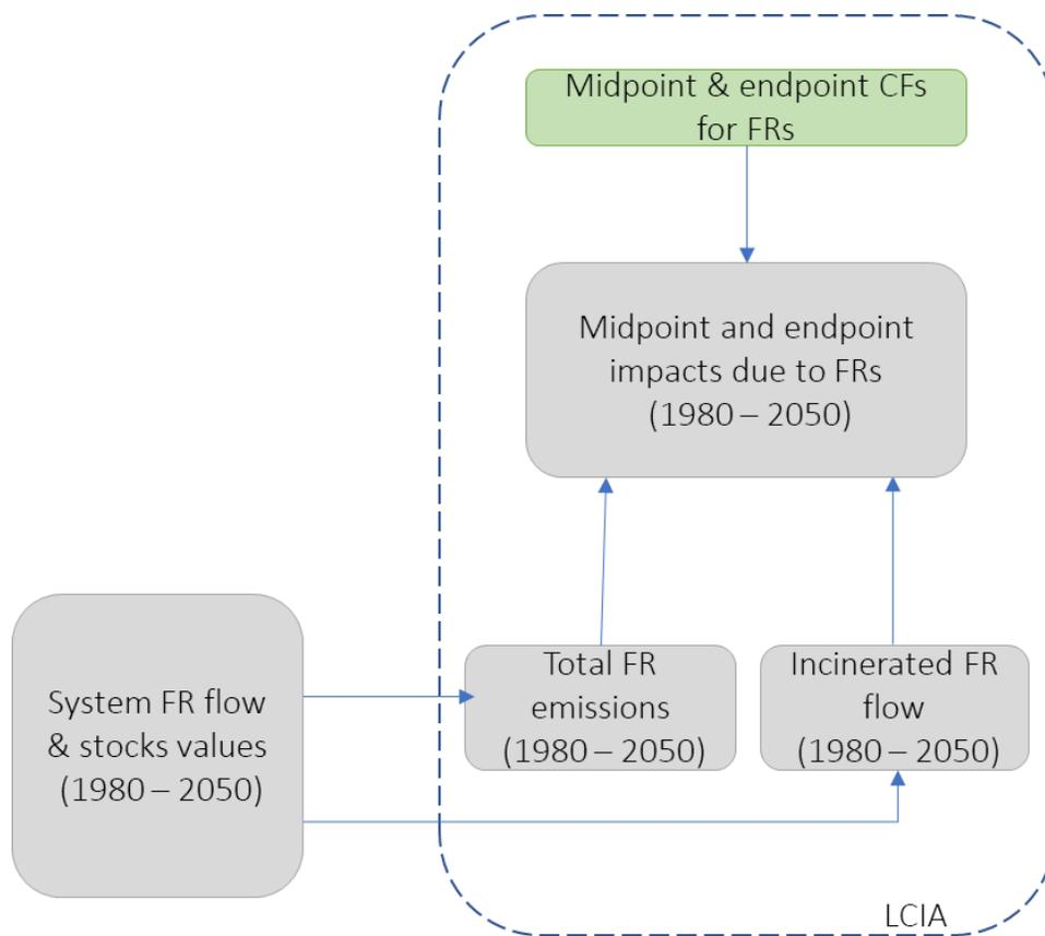
Figure 2.7. An overview of the steps required to get to the midpoint and endpoint impact results, linking the LCIA method with the flame retardant flows resulting from the layered dynamic MFA.
