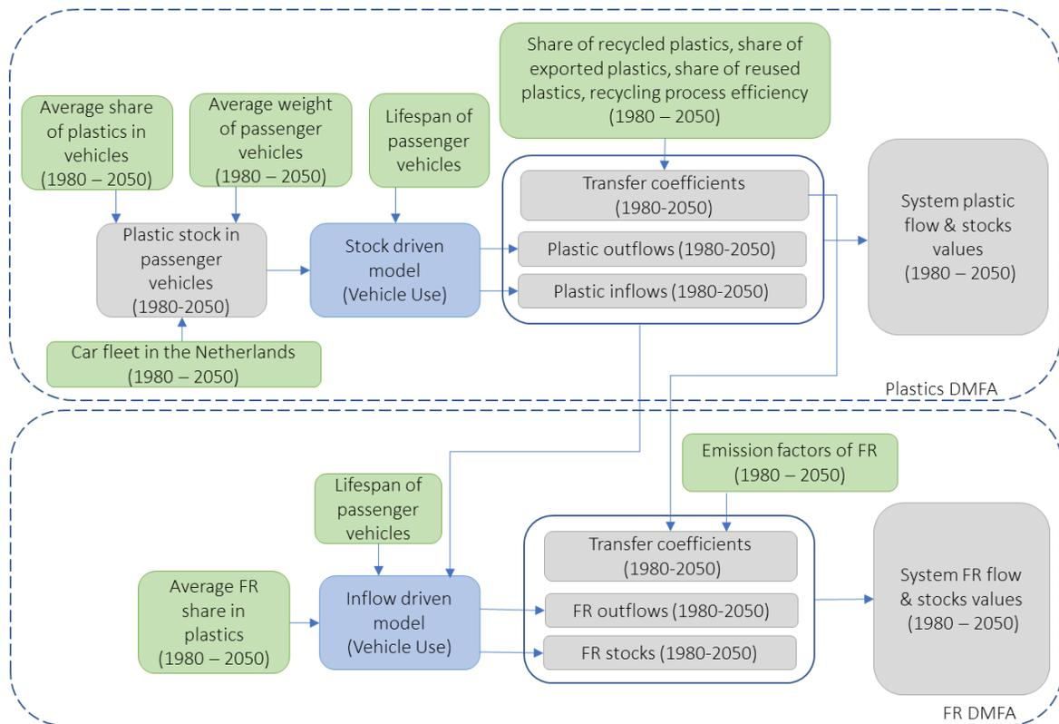
Figure 2.5. Overview of the required data and calculation steps to determine the plastic and FR system flows from 1980 through 2050. Green boxes indicate required data, light grey boxes indicate calculated values.
