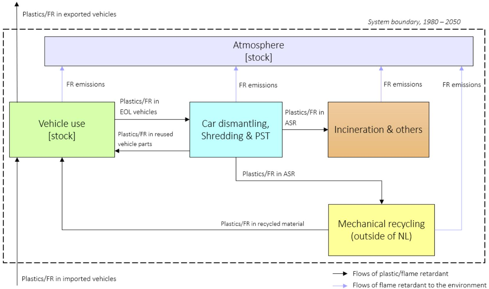
Figure 2.4. Defined system for plastics, decaBDE and TPP in the time-period 1980 – 2050 (needs update to add flow from mechanical recycling to incineration and put atmosphere outside the system boundaries).
