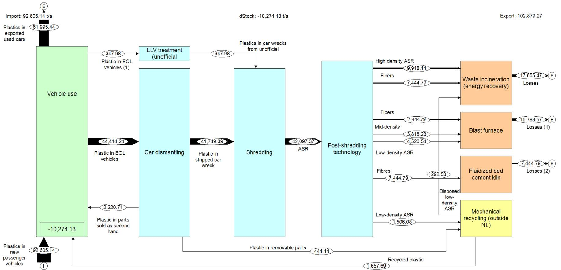
Figure 3.1. Quantification of plastics in passenger vehicles in The Netherlands in 2019 (unit: tons/year).
