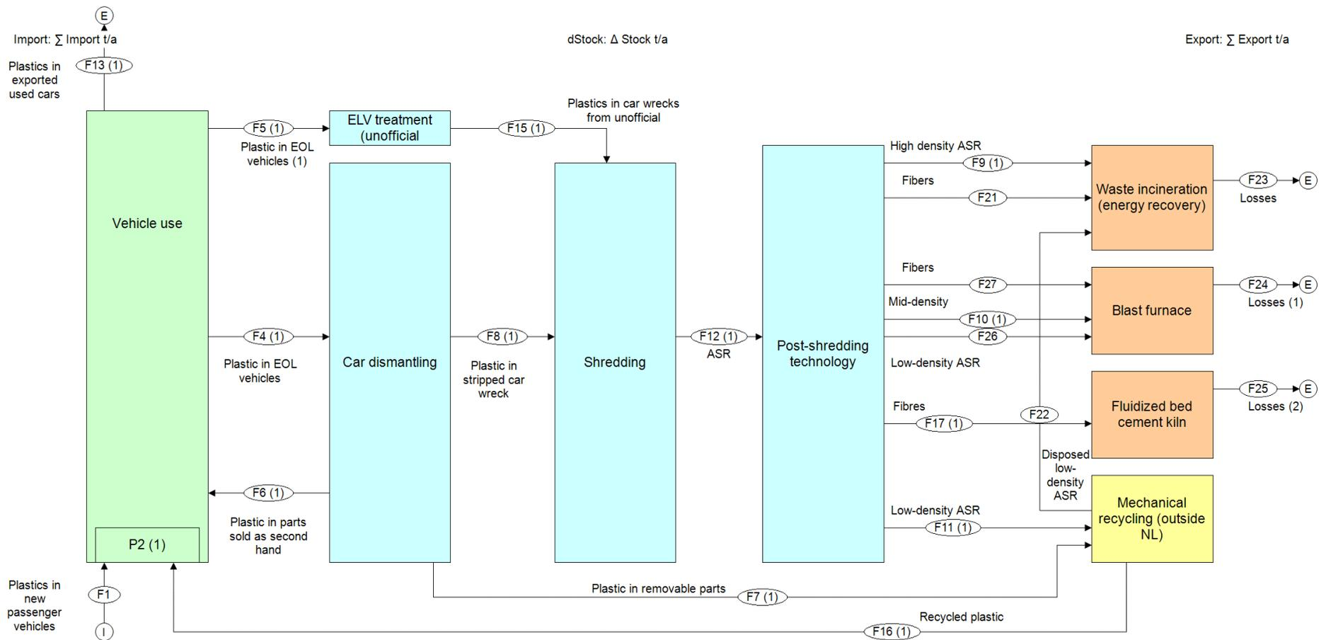
Figure 2.1. Graphical representation of the system of the material flow analysis for plastics in passenger vehicles in The Netherlands in 2019.
