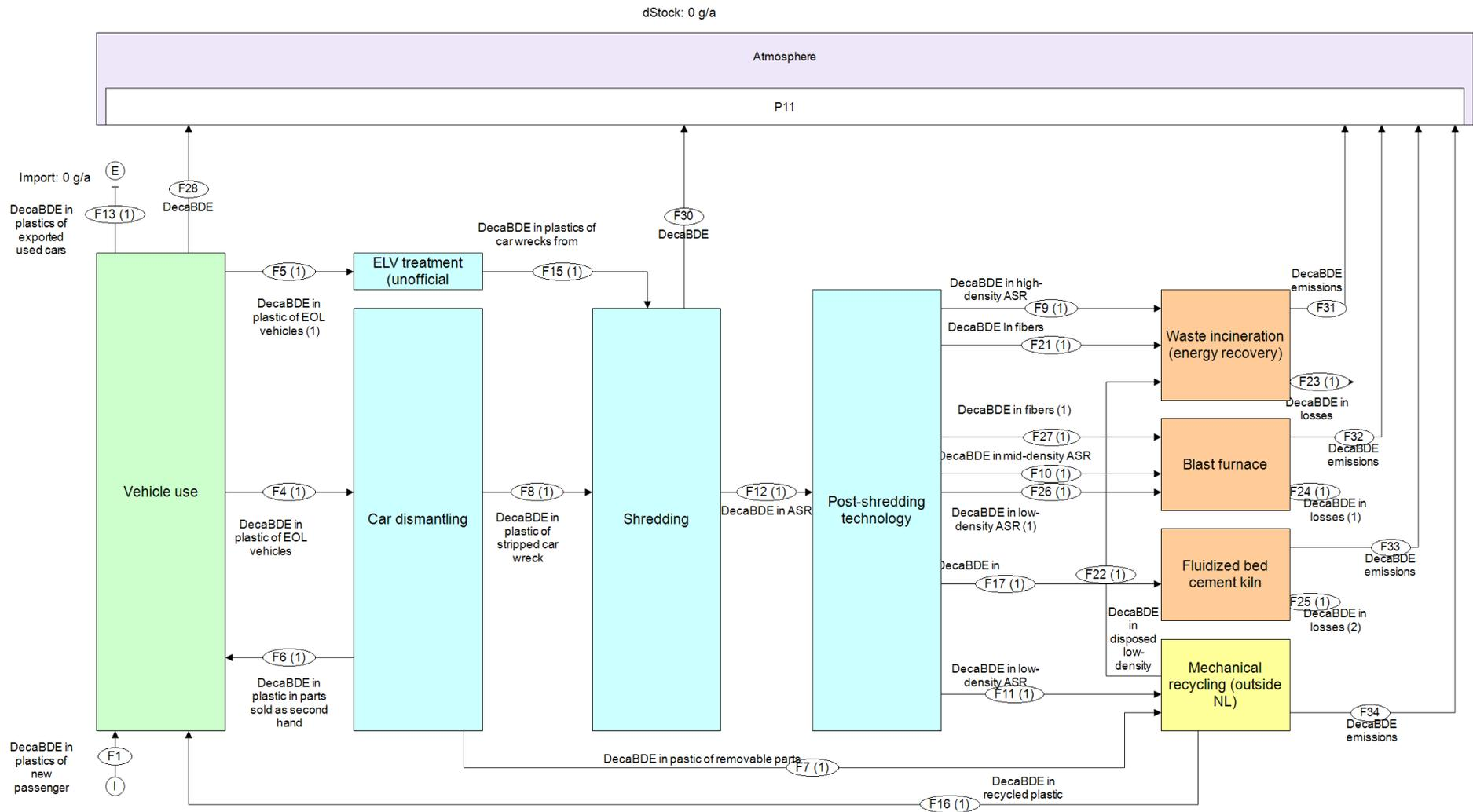
Figure 2.2. Graphical representation of the system of the static material flow analysis for decaBDE in plastics of passenger vehicles in The Netherlands in 2019.
