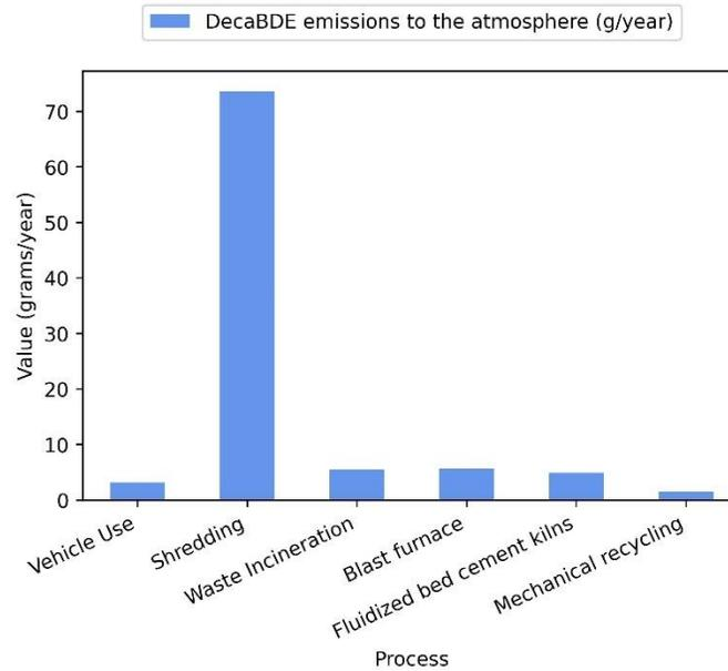
Figure 3.5. DecaBDE emissions to the atmosphere per process according to the static decaBDE MFA (unit: grams/year).
