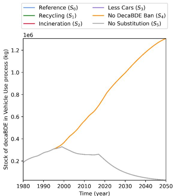
Figure 3.9. Stock of decaBDE in Vehicle Use process.
