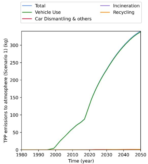
Figure 3.15. TPP emissions to atmosphere per process for the Recycling scenario (S1).
