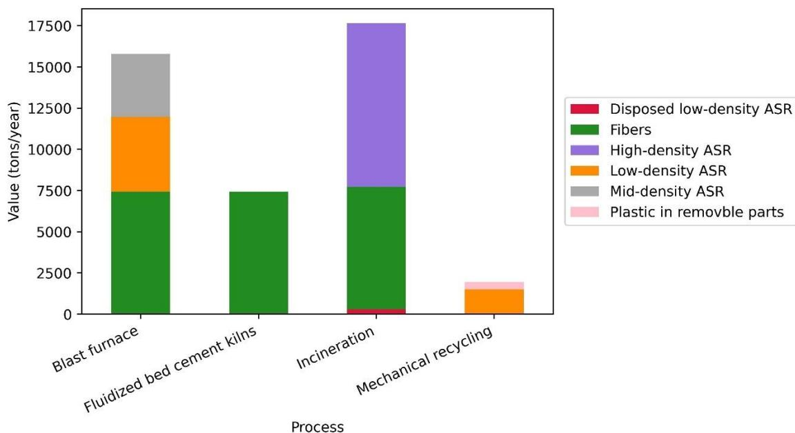
Figure 3.3. Stacked bar plot of the main destinations of ASR plastics after exiting the Post-Technology Shredder process. Each bar represents total amount of plastics destined to each process. Within each bar, distinctions are made between the types of plastics flows that are destined to the process.
