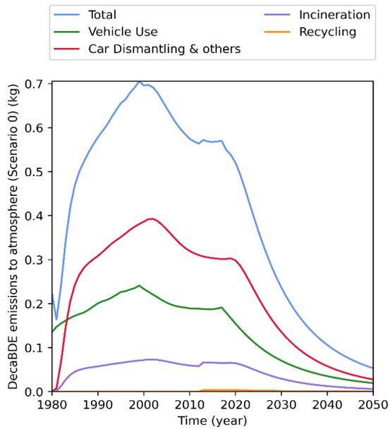
Figure 3.13. DecaBDE emissions to atmosphere per process for the Reference scenario (S0)
