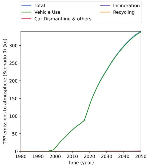
Figure 3.16. TPP emissions to atmosphere per process for the Reference scenario (S0).
