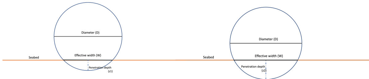
Figure A.1: Visualization of effective width
