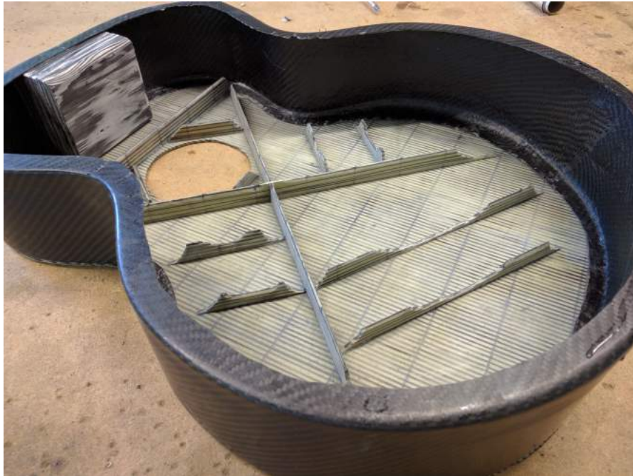
Figure 22.3: Final shape of the braces after material was removed in several iterations to improve acoustic response.
