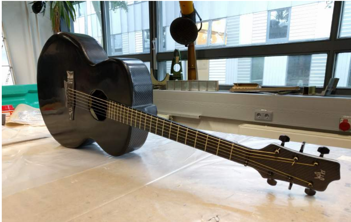
Figure 24.3: The composite guitar with strings attached and final finishing and set-up completed.
