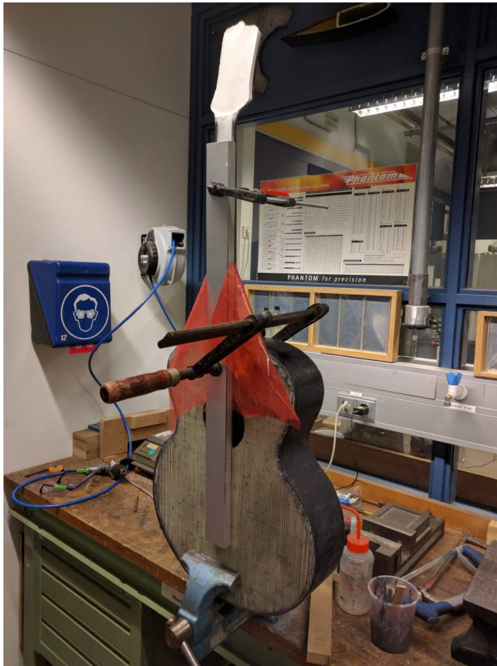
Figure 23.1: Installation of neck to the body using a straight rectangular profile clamped to the neck and body.
