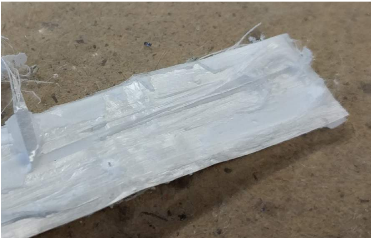
Figure 12.3: Photo of the inner surface of the second failed sample. The splitting of the Endumax tape through its thickness is clearly visible.
