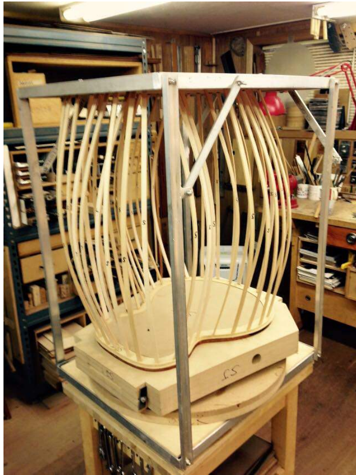
Figure 20.2: Table with a specific radius used to create a slightly double curved and pre-tensioned soundboard [34]
