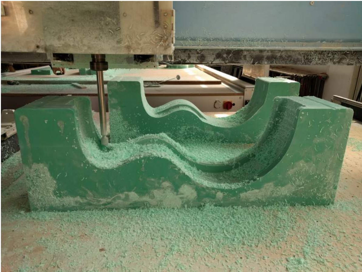
Figure 21.7: Pre-milling of the sides mould with an elongated CNC mill.
