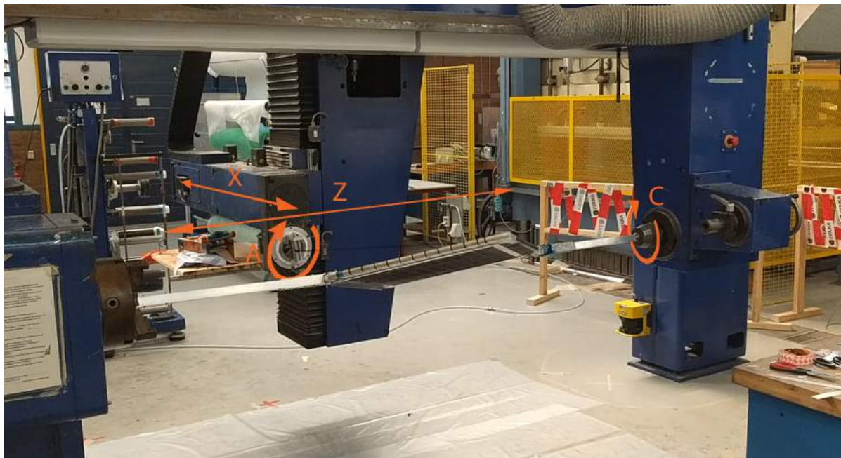
Figure 14.2: Photo of the filament winding set-up on which each of the axes are indicated.
