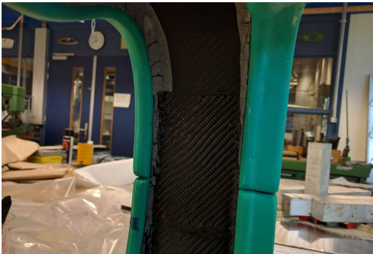
Figure 22.8: Application of a small patch of wetted carbon fibre fabric to bond the two side pieces.
