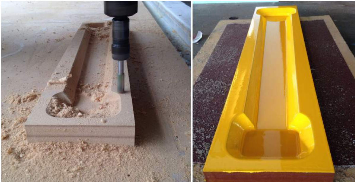
Figure 21.2: Left: CNC milling of fretboard mould out of MDF. Right: first fretboard mould version after application of Doublecoat lacquer.
