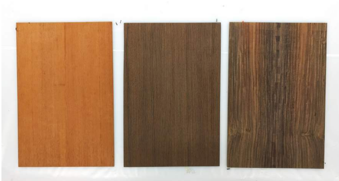
Figure 11.4: Back and sides woods investigated. From left to right: mahogany, wenge, East-Indian rosewood.
