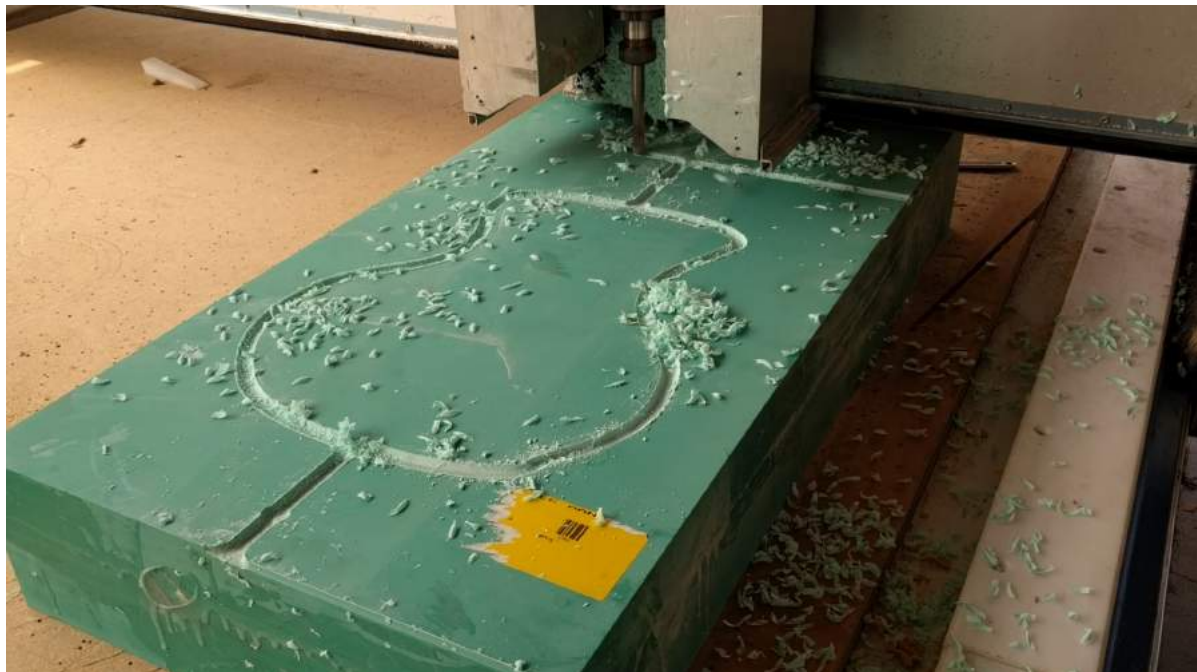
Figure 21.6: Contour milling of the sides mould out of bulk Sikablock M945
