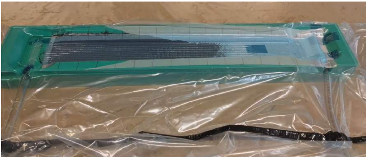
Figure 21.3: Second version of the fretboard mould milled from Sikablock M945 tooling block. The infusion inlet is created on the left side. The exit towards the vacuum pump is on the right side.
