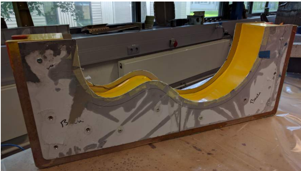
Figure 21.4: Upper component of the produced sides mould including the aluminium panels.
