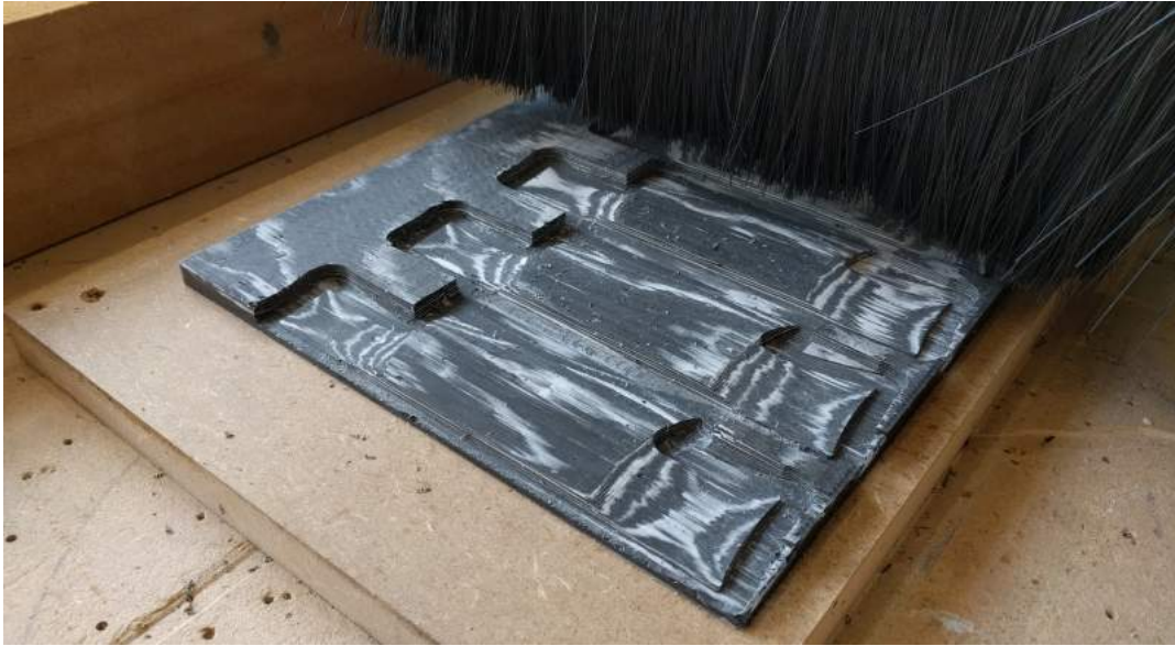
Figure 22.16: Milling of the contour of the bridges up to 1 mm above the bottom surface of the blank.
