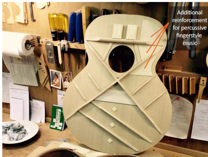
Figure 2.9: Fingerstyle guitartop by Marc Beneteau showing the additional patches to reinforce the soundboard against the impact of percussion on the guitar body [34].
