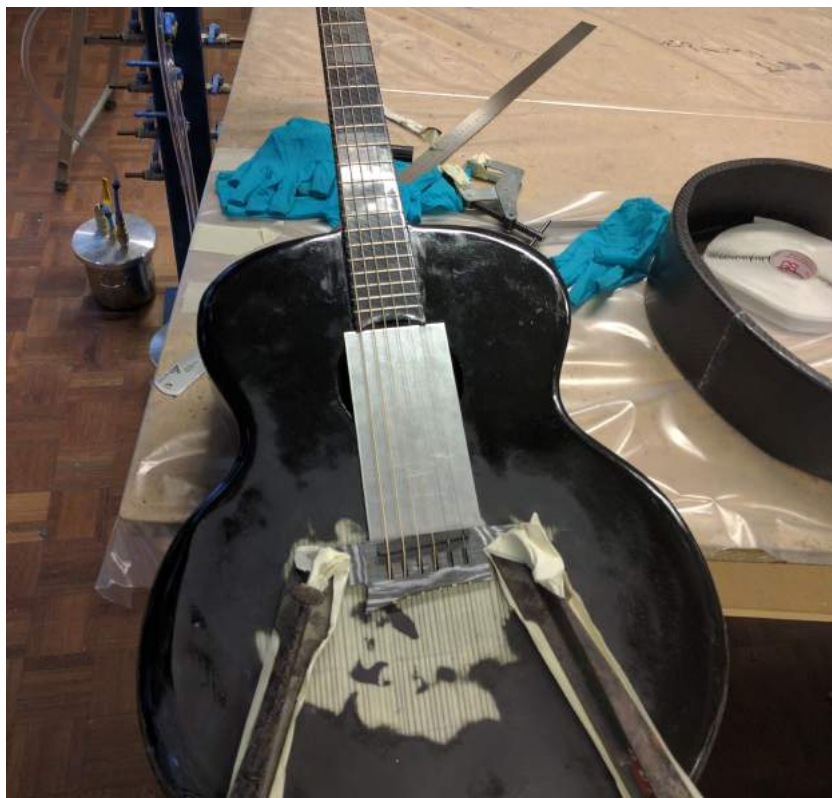
Figure 24.2: Process of finding the optimal bridge position for intonation using an aluminium plate and two large clamps.
