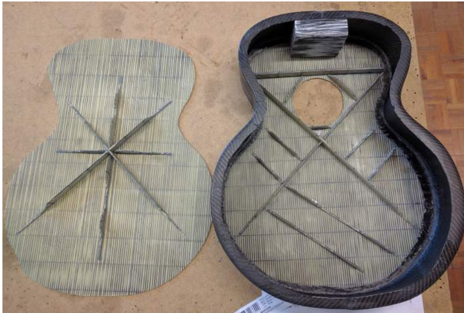
Figure 22.4: Left: Back with braces attached and finalized to desired shape. Right: Soundboard assembled to the sides.
