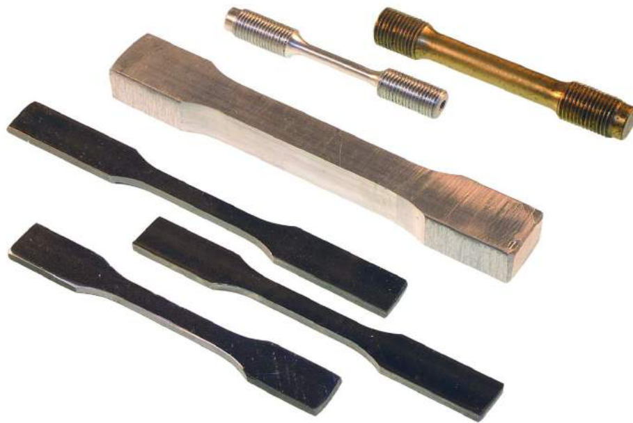
Figure 5.1: Dogbone shaped test samples for the determination of stiffness and strength of a material [57]
