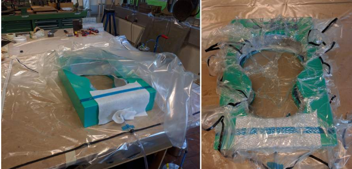
Figure 22.9: Construction of a large vacuum bag around the product. Left: the vacuum bag before vacuum is applied. Right: the vacuum bag after application of vacuum
