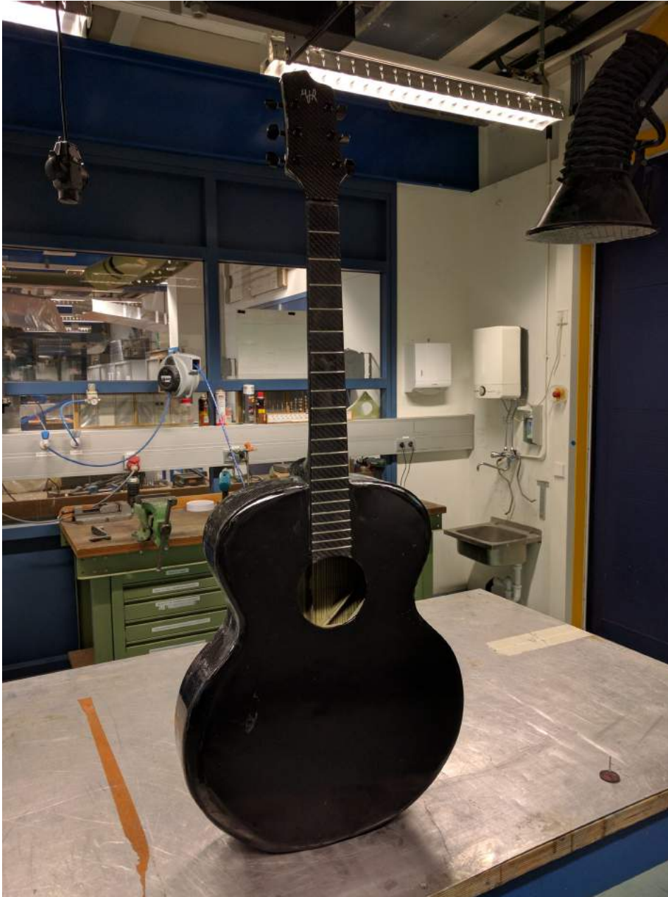
Figure 23.2: Assembly of the guitar components before installation of the bridge, nut and saddle.
