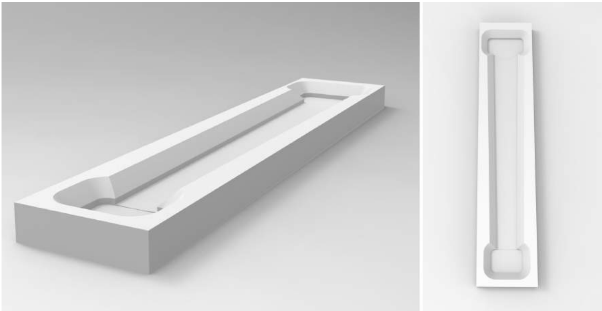
Figure 21.1: Rendering of the first version of the fretboard mould. Isometric view (left) and top view (right)
