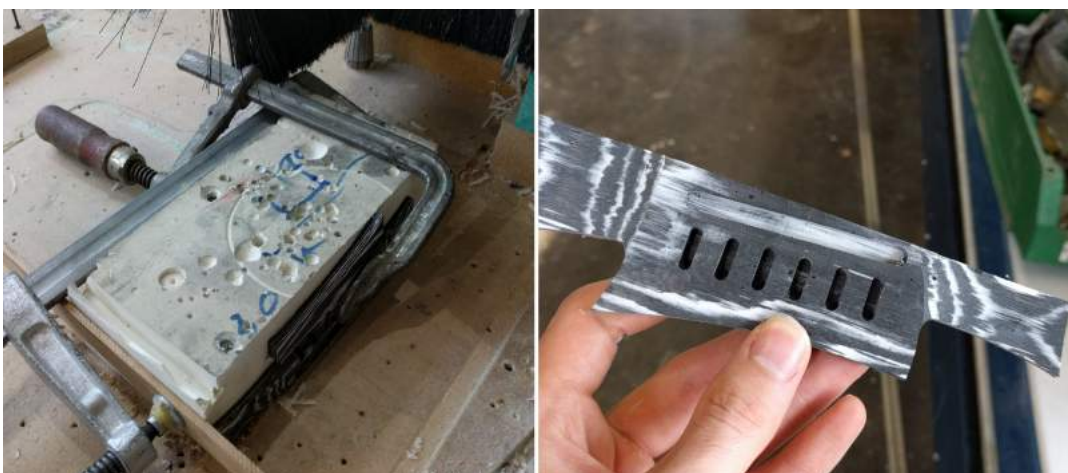
Figure 22.17: Left: bridge constrained at its side for the milling of small holes on the back side of the bridge. Right: completed bridge.
