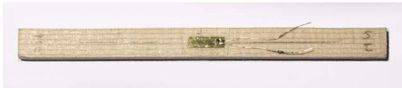
Figure 10.1: Strain gauge attached to a master grade sample (MA-L-4) used for the determination of stiffness.
