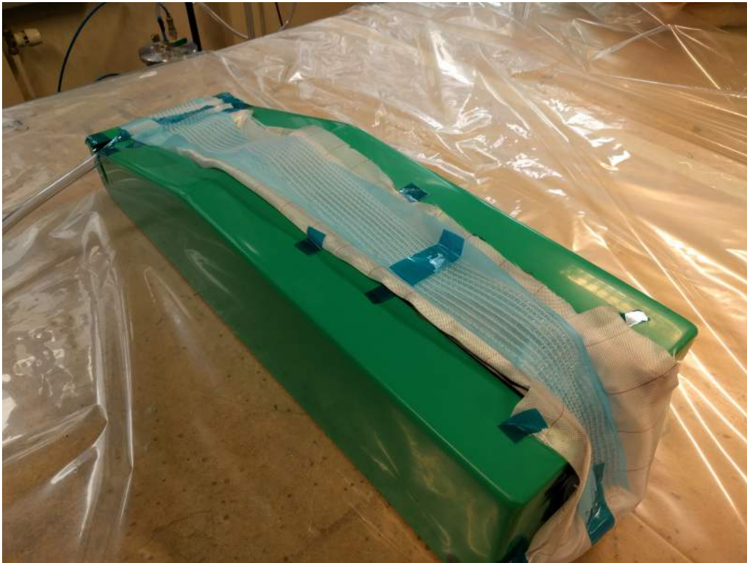
Figure 22.12: Lay-up of infusion materials before the vacuum bag is closed and vacuum is applied.
