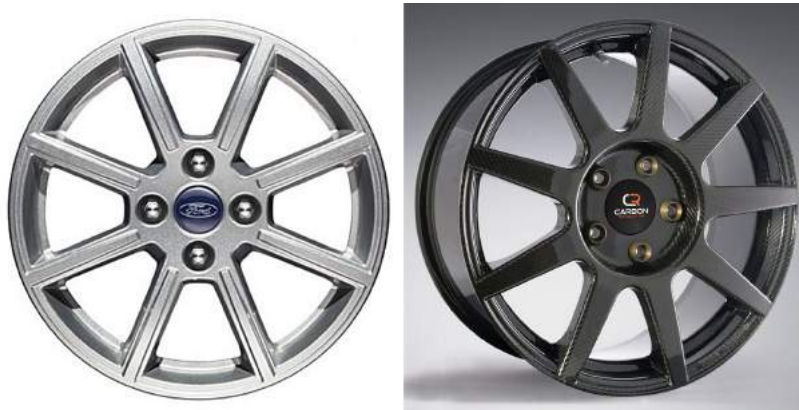
Figure 6.3: Two eight spoke car rims. Left: Aluminium rim, Right: Carbon fibre reinforced polymer rim. [94, 95]
