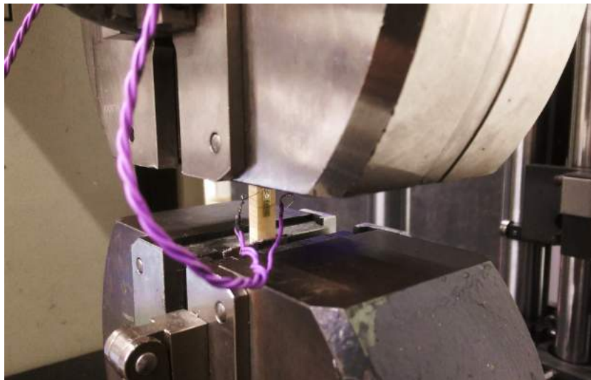
Figure 10.2: Wood sample set-up in the Zwick 20kN testing machine with the strain gauge attached to the Wheatstone bridge amplifier.
