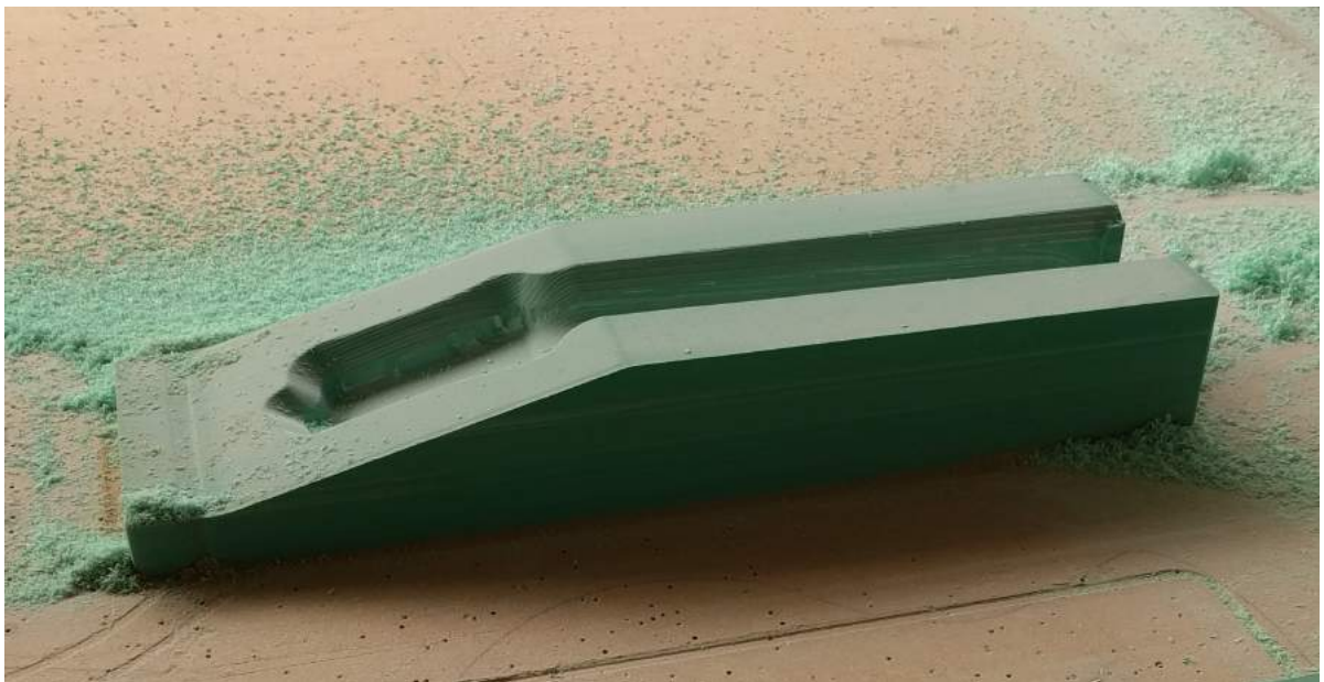
Figure 21.11: Pre-milling of the 100 mm block which would later be glued on top of the 50 mm block.
