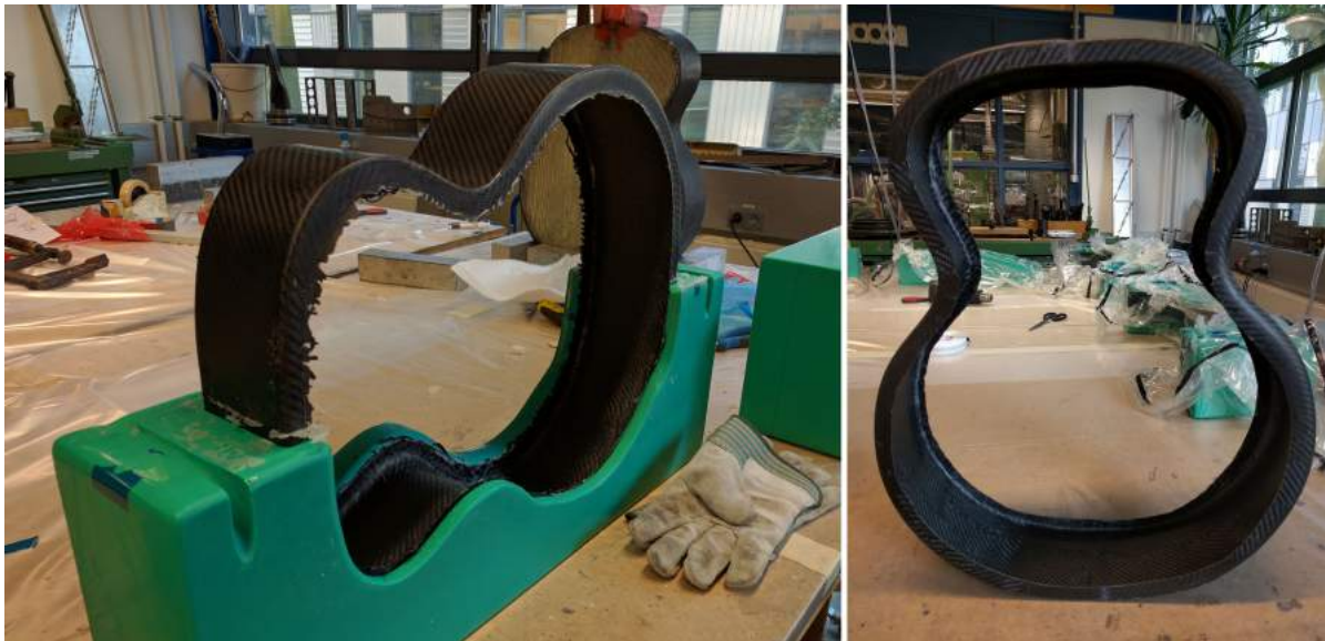
Figure 22.10: Left: de-moulding of the sides. Right: the sides after trimming with a dremel hand tool.
