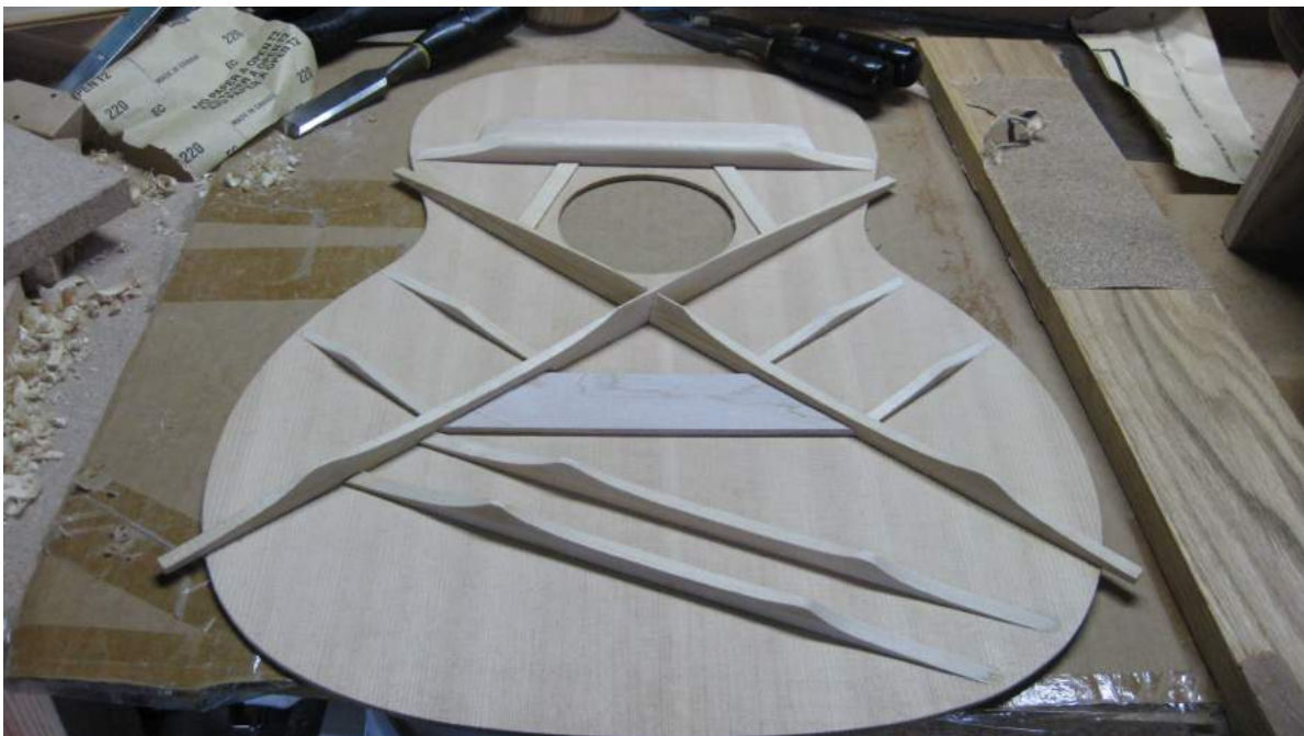
Figure 2.3: Martin & Co. x-brace style bracing pattern used for most acoustic steel string guitars [19].
