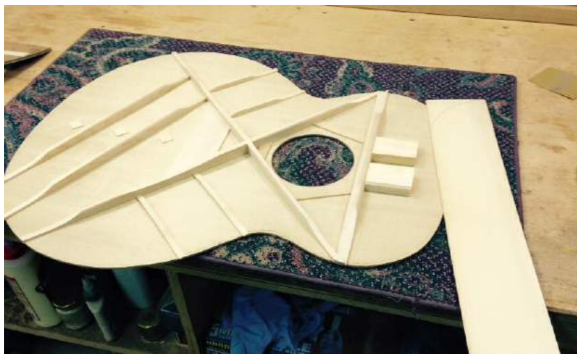
Figure 3.1: Barcing pattern of a modern fingerstyle steelstring acoustic guitar by Marc Beneteau [34]
