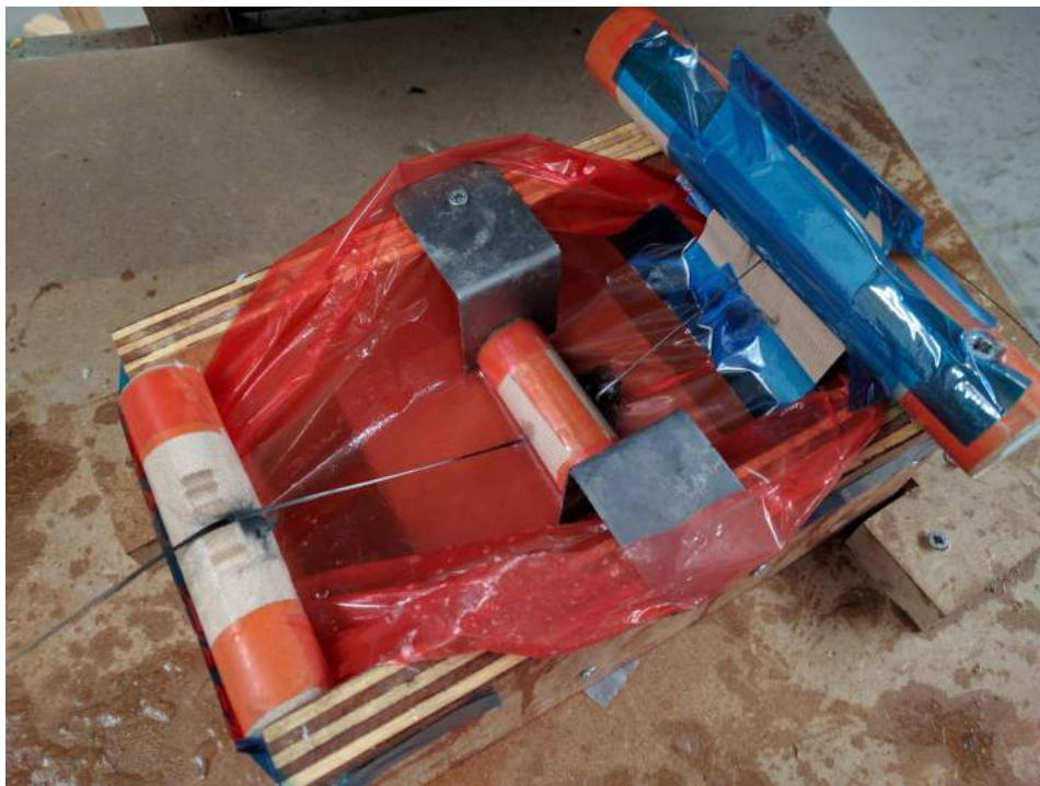
Figure 14.6: Fibre wetting device which applies a small amount of epoxy resin to the filament. At the entrance point of the device a small amount of loose carbon fibre material builds up during the plate winding process.
