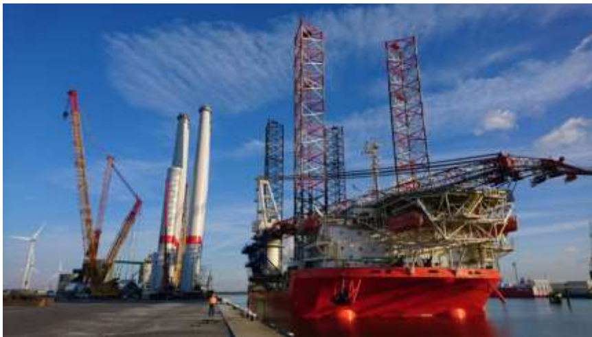
Figure 1-1 Seafox 5 in the harbour with the wind turbines towers on quayside to be loaded
