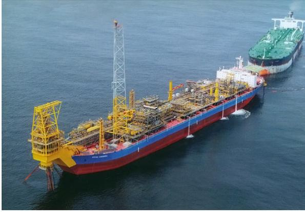
Figure 1.1: Tandem offloading FPSO Xibomba
