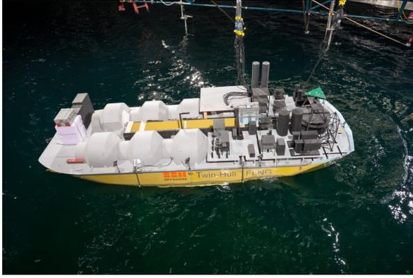
Figure 4.4: Twin Hull in Offshore Basin at MARIN
