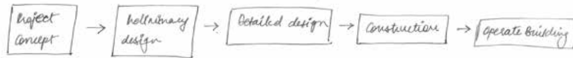
Fig 5.1.2.a: Design -Build project delivery phases. Based on text from (Cushman et al, 2001). (Illustration by self)
