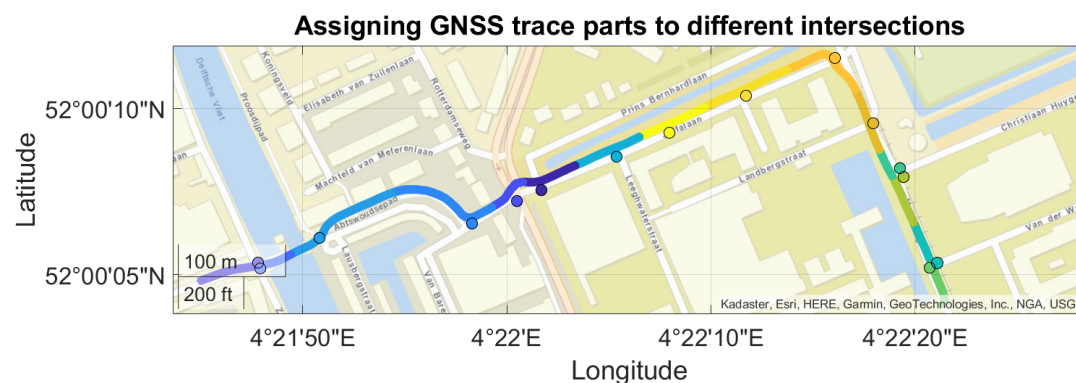
Figure 2.8: Separating parts of the GNSS trace based on proximity to intersections. Each different color of the GNSS trace corresponds to a different intersection. Intersection geolocations are shown as colored circles with a black perimeter.
