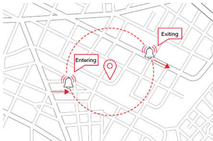
Figure 1.7: An example of the practical implementation of a geofence. The geofence could correspond to a low-speed e-bike area, where the cyclist will not be assisted by the motor of the e-bike, for example.
