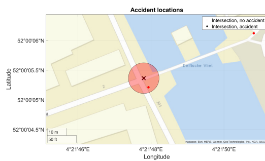
(c) Map view of Figure 2.6a. Since the bottom geolocation is within 8 meters of the dangerous intersection, the accident counts for both geolocations are combined. If a cyclist would cross the intersection, the analysis will now show consistent results when the cyclist GNSS trace is linked to either geolocation, as both geolocations now share their accident counts.
