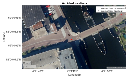
(a) Two geolocation entries in the digital road network for one actual intersection. One geolocation has accidents linked to it (black cross), but the other geolocation (red dot) has no accidents associated with it. If a cyclist would cross this intersection, the cyclist GNSS trace could be linked to either one of these geolocations since they are extremely close together. To make sure that the analysis shows consistent results, the accidents counts of both locations are combined.
