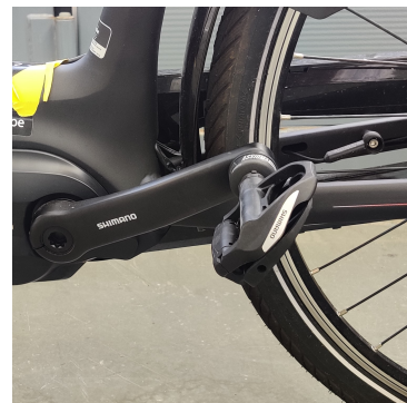
(d) The regular pedals have been replaced by power meter pedals (Favero Assioma DUO). The power data is logged with a cycling app on the phone during the experiment.
