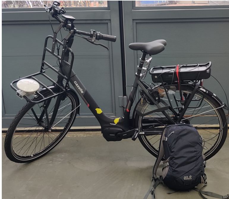
(a) The e-bike (Gazelle Grenoble C8 HMS prototype e-bike) used during the natural cycling experiment, along with the attached sensors. The backpack contains the evaluation board of the GNSS antenna.
