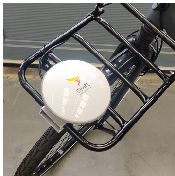
(c) Front rack carrying the GNSS antenna of the Piksi Multi GNSS module. The evaluation board (along with the USB logging device and power supply) is placed in the backpack, which is connected to the antenna with a wire running along the bicycle frame.
