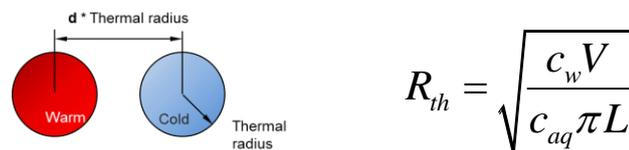
Figure 5. ATES well layout and footprint definition. Thermal radius depends on thermal properties of aquifer and water ( $c_{aq}$ ,  $c_w$ ), storage volume ( $V$ ) and filter screen length ( $L$ )
