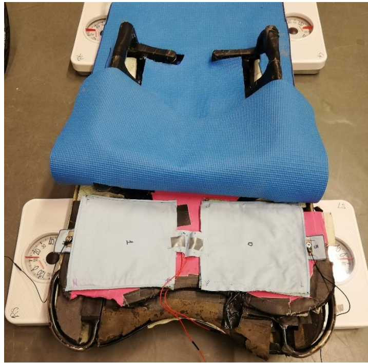
Figure 2.24. Placement of the sensors.
