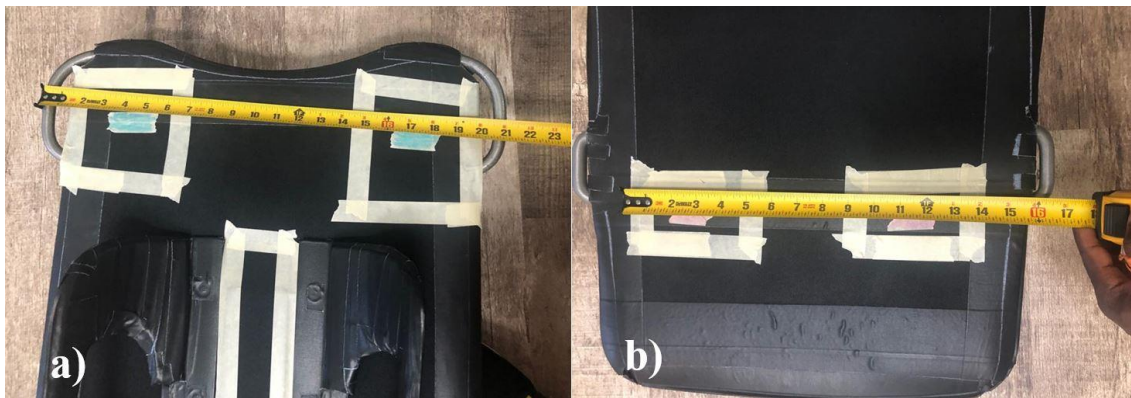
Figure 2.6. The dimension of the sensors. In figure a) and b) it is shown an approximation of the size of the sensors for the shoulders and the knees respectively sent by the athlete. The metric tape is in inches.
