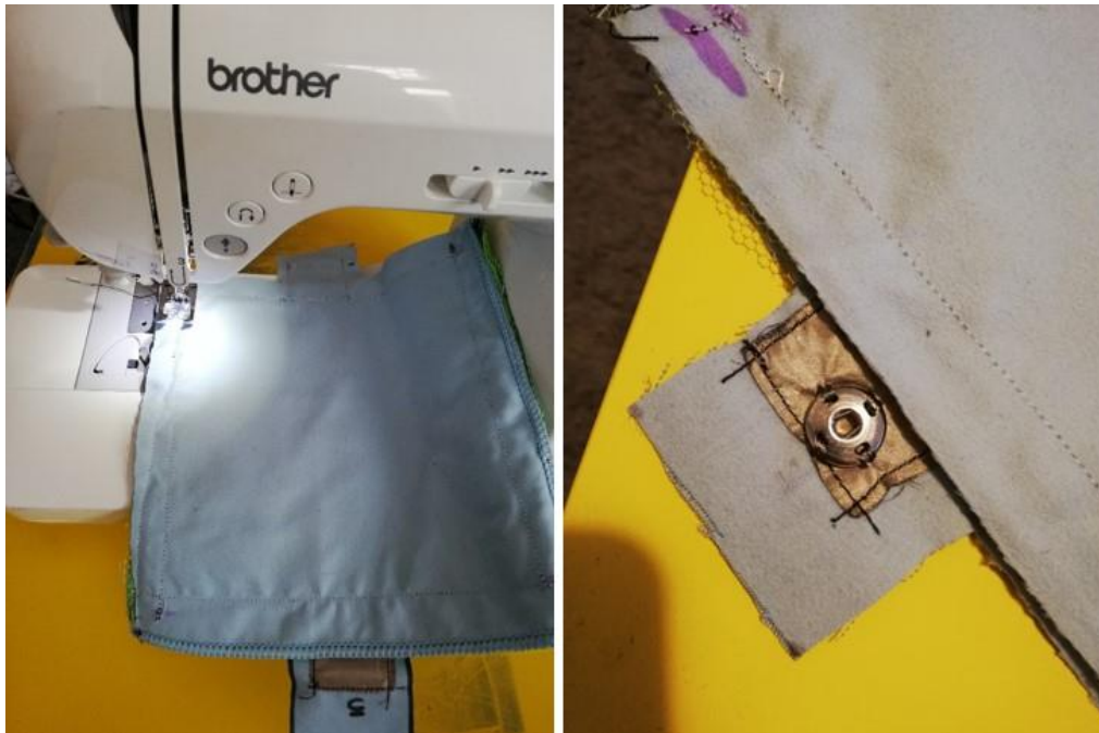
Figure 2.19. Last steps of the manufacturing of the sensors. In the left picture, the sensor is being sewed together and in the right one, the metallic button is attached.
