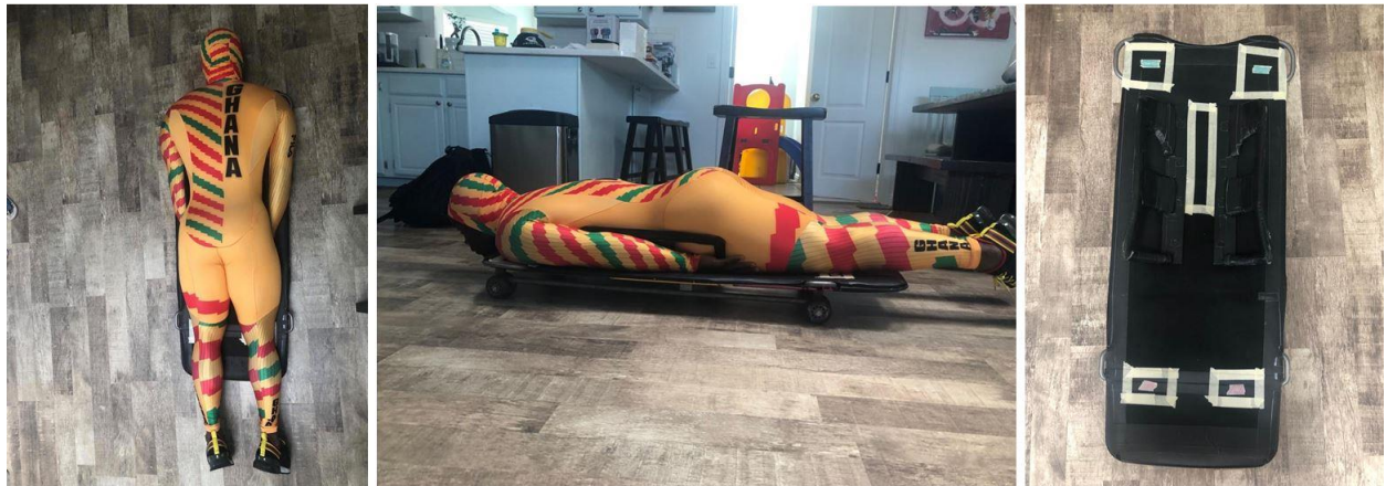
Figure 2.25. Akwasi Frimpong position on the sled. Shoulders and knees location to put the tactile force sensors.
