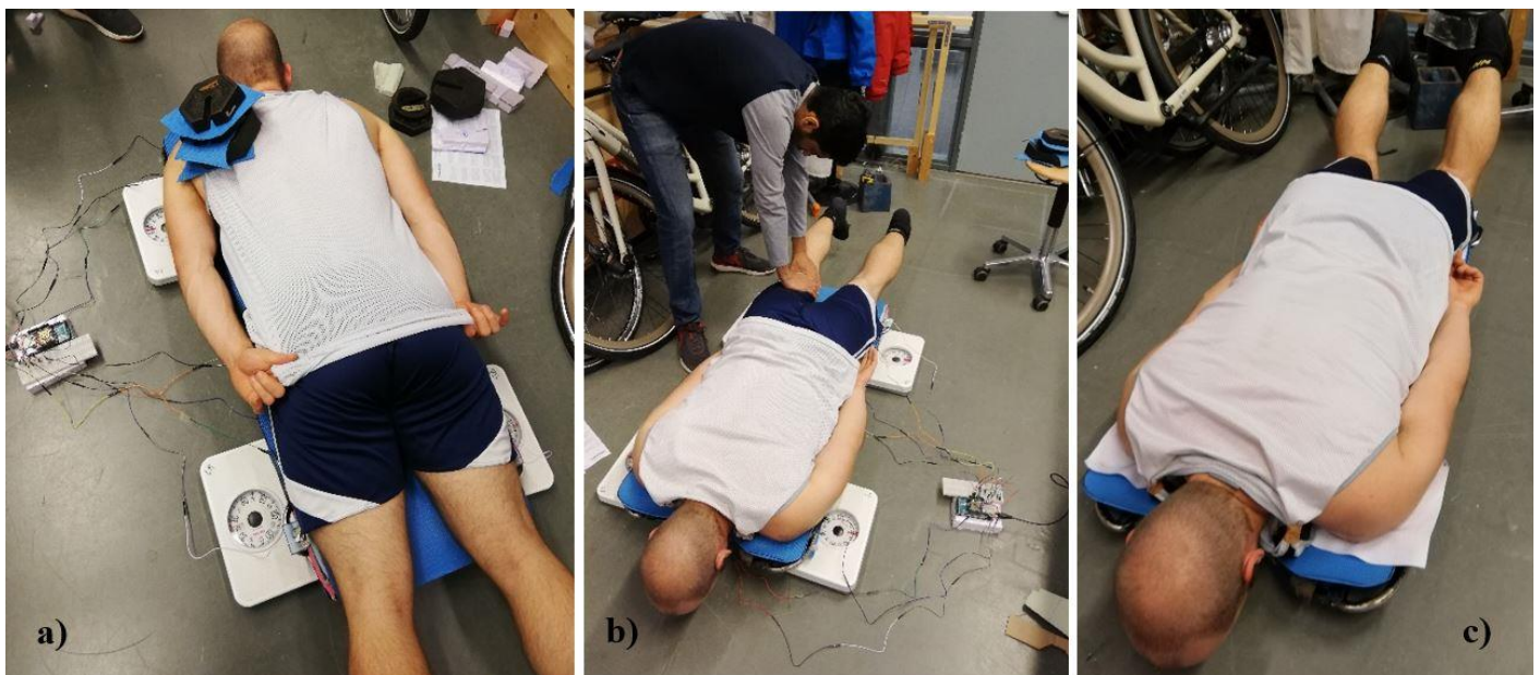
Figure 3.2. Tests accomplished. a) Fixed weights on top of each joint, b) Constant force applied by someone, c) Free steering forces applied.
