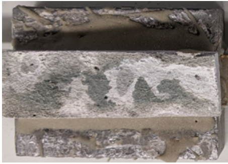
Figure D.19: Bottom debonded part of Specimen TG20-A-3
