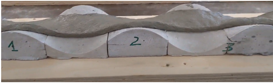
Figure 4.8: Casting of first layer using caulk-gun on the base blocks (Positions 1, 2, 3 indicate the positions at which samples were sawn at a later stage for further testing)
