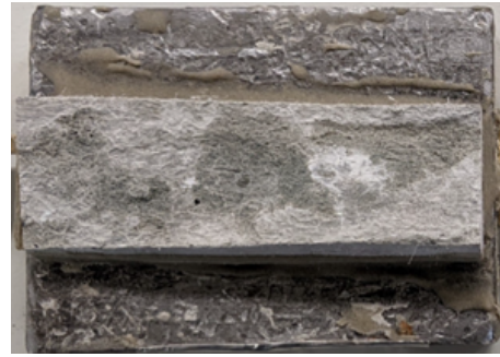
Figure D.4: Top debonded part of Specimen TG5-A-3
