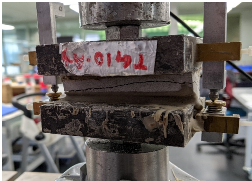
Figure C.7: Specimen TG10-A-4 after failure
