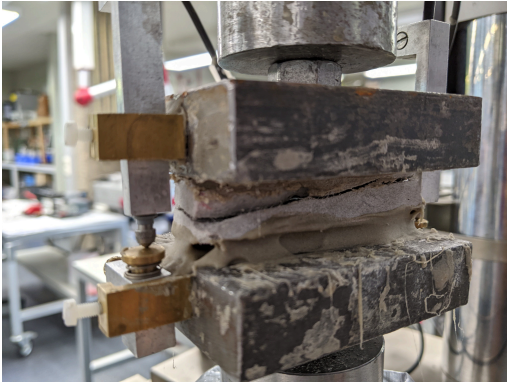
Figure C.14: Specimen TG5-B-3 after failure
