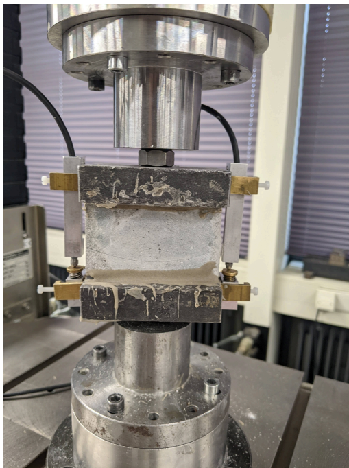
Figure C.43: Casted Specimen C-3 after failure
