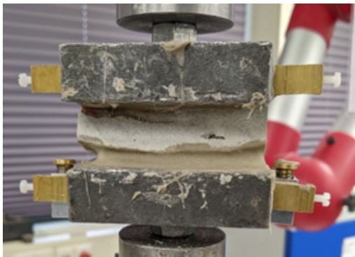
Figure 5.8: Specimen TG20-B-3 after failure: The thickness of the upper layer is less as compared to bottom extruded layer
