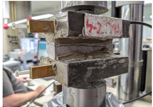
Figure C.27: Specimen TG5-C-4 after failure
