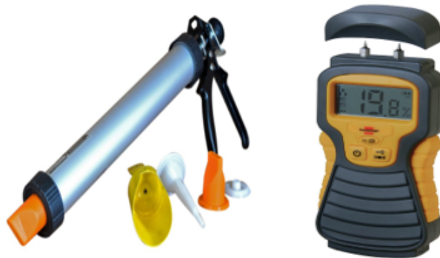
Figure 4.2: (Left) Roughneck mortar gun used for scale model 3D concrete printing for extrusion (Right) Brennenstuhl 1298680 Moisture meter MD
