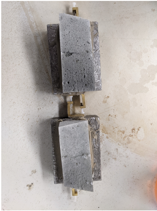
Figure D.75: Inter-layer surface of Casted Specimen C-2 after failure
