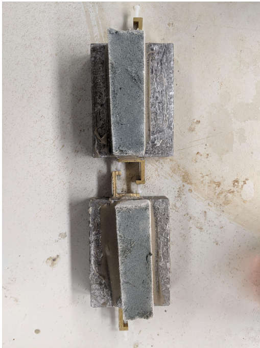
Figure D.77: Inter-layer surface of Casted Specimen C-4 after failure
