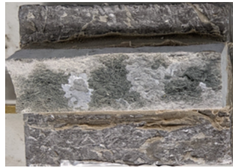
Figure D.14: Top debonded part of Specimen TG10-A-4
