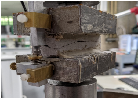
Figure C.5: Specimen TG10-A-2 after failure
