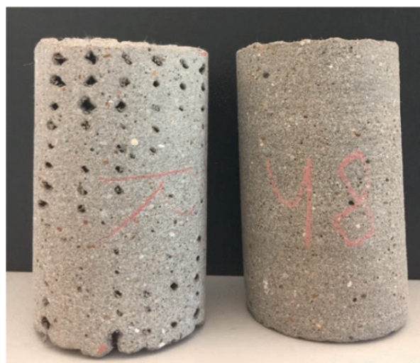
Figure 1.1: (Right) Good quality sample with an identifiable outline of each filament, interspersed with voids (Left) Poor quality sample with the indiscernible filaments [1]
