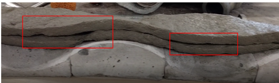
Figure 5.12: Extruded second layer on the first layer (Regions highlighted with red show defects in the specimens related to non-uniform contact between layers and non-uniform layer thickness induced due to the caulk gun extrusion process)
