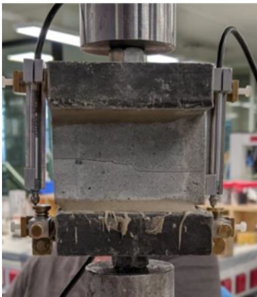
Figure C.39: Casted Specimen B-3 after failure
