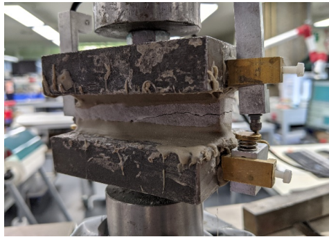
Figure 5.25: Failure of Specimen TG5-C-3 influenced by asymmetry (bottom layer)
