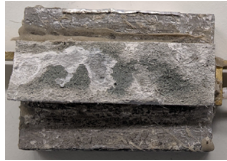
Figure D.20: Top debonded part of Specimen TG20-A-3
