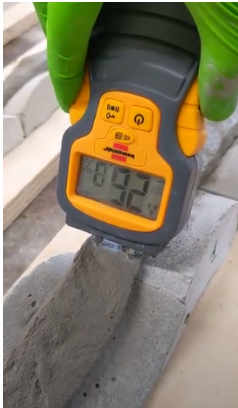
Figure 4.9: Measurement of surface moisture content on the first extruded layer using moisture measuring device
