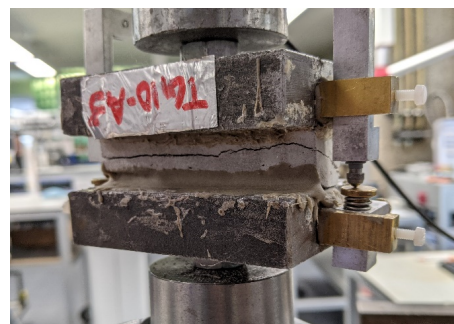
Figure C.4: Specimen TG10-A-3 after failure
