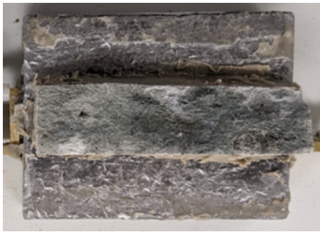
Figure D.29: Bottom debonded part of Specimen TG5-B-4
