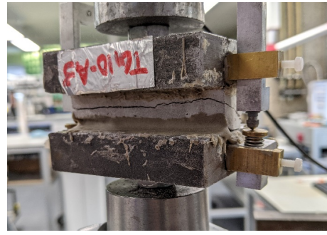
Figure C.6: Specimen TG10-A-3 after failure
