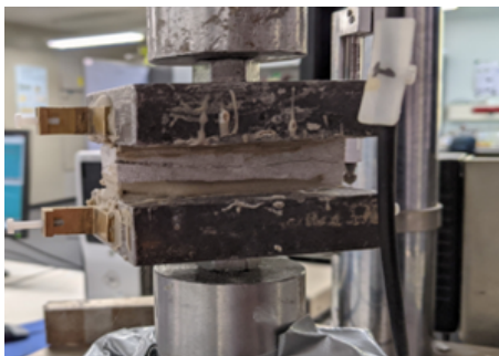
Figure C.1: Specimen TG5-A-2 after failure
