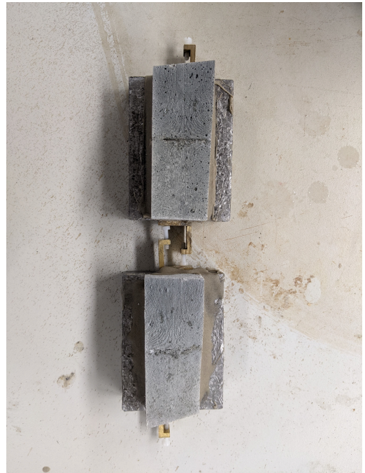
Figure D.70: Inter-layer surface of Casted Specimen A-4 after failure
