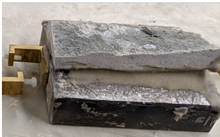
Figure D.37: Bottom debonded part of Specimen TG10-B-4
