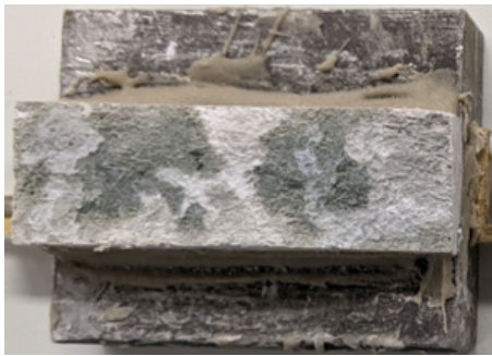
Figure D.9: Bottom debonded part of Specimen TG10-A-2
