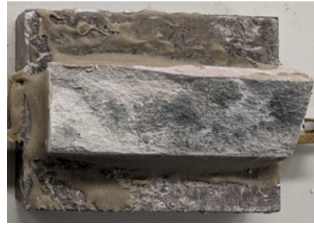
Figure D.64: Top debonded part of Specimen TG20-C-3
