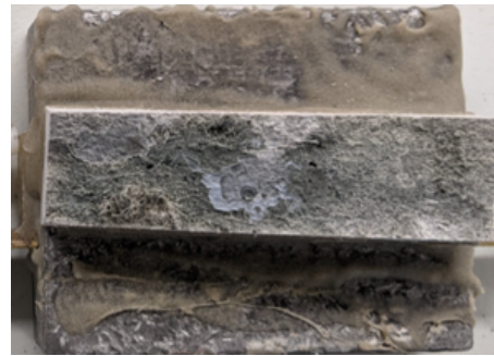
Figure D.30: Top debonded part of Specimen TG5-B-4
