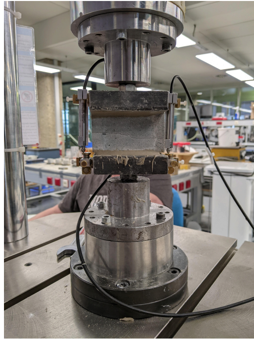
Figure C.38: Casted Specimen B-2 after failure
