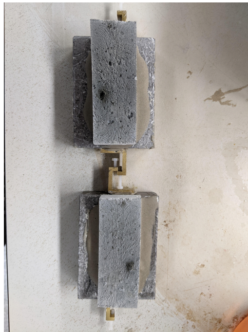
Figure D.72: Inter-layer surface of Casted Specimen B-3 after failure
