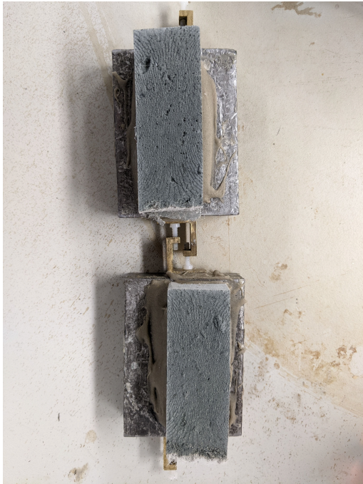
Figure D.67: Inter-layer surface of Casted Specimen A-1 after failure
