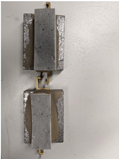
Figure D.73: Inter-layer surface of Casted Specimen B-4 after failure
