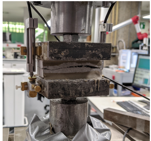
Figure C.17: Specimen TG10-B-2 after failure
