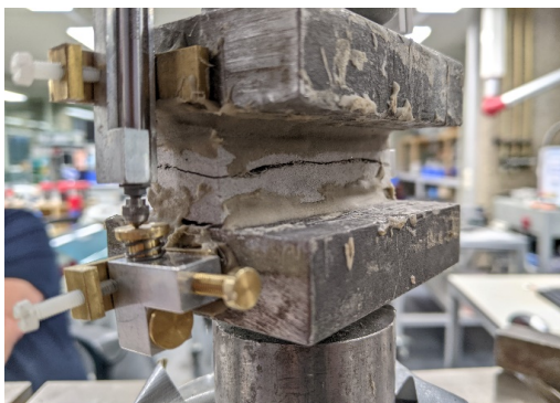
Figure C.28: Specimen TG10-C-2 after failure
