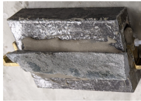
Figure D.46: Top debonded part of Specimen TG20-B-4
