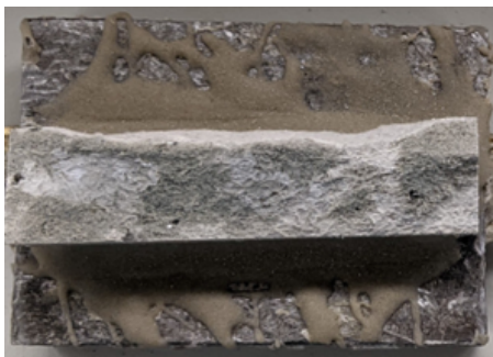
Figure D.1: Bottom debonded part of Specimen TG5-A-2
