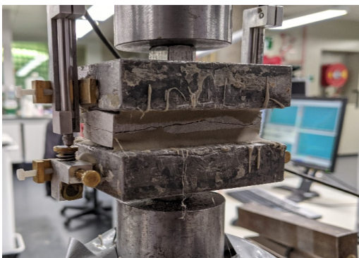
Figure C.20: Specimen TG20-B-1 after failure
