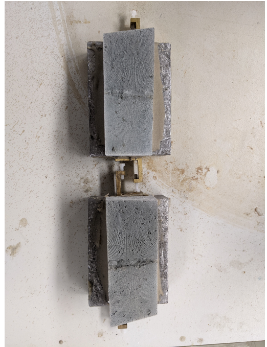
Figure D.68: Inter-layer surface of Casted Specimen A-2 after failure
