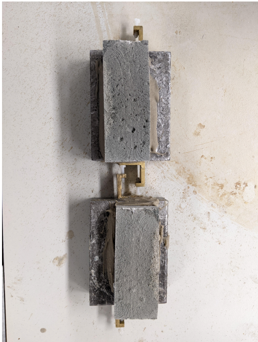
Figure D.69: Inter-layer surface of Casted Specimen A-3 after failure
