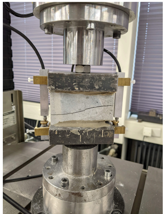
Figure C.44: Casted Specimen C-4 after failure
