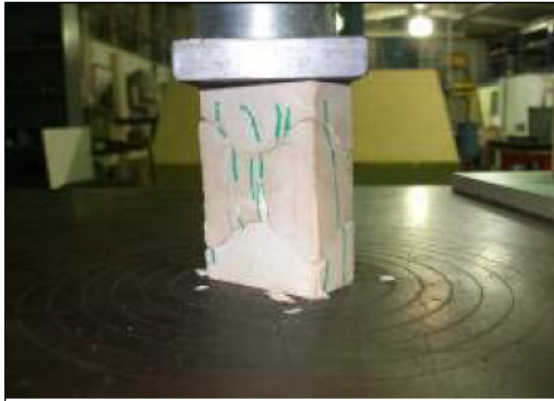
Figure 2.42: Assembly of Osteomorphic block for axial compression test [47]
