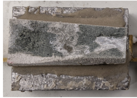
Figure D.40: Top debonded part of Specimen TG20-B-1
