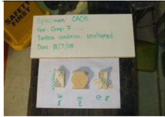
Figure 2.43: Identification of crack formation in the osteomorphic block after compression test [47]
