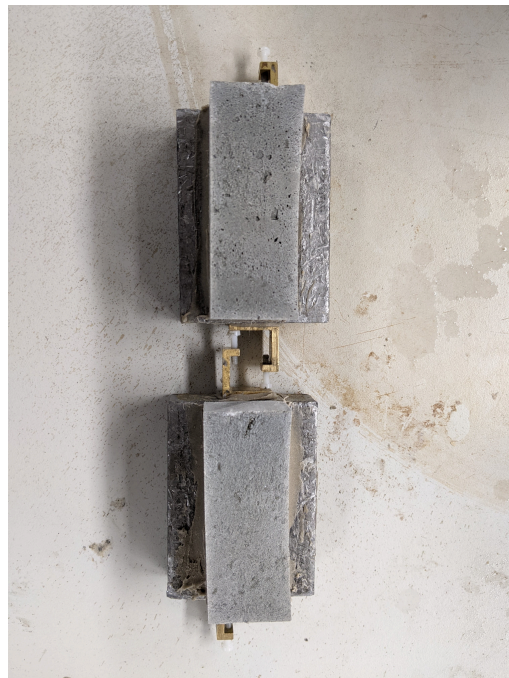
Figure D.74: Inter-layer surface of Casted Specimen C-1 after failure
