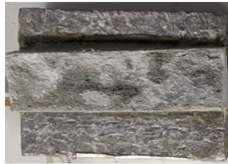
Figure D.6: Top debonded part of Specimen TG5-A-4
