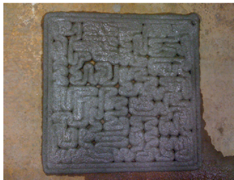
Figure 2.8: Under-filling due to nozzle direction change [1]
