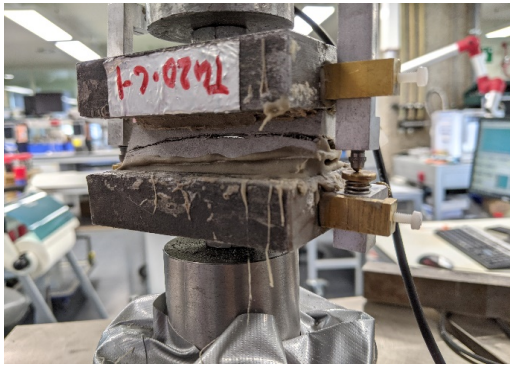
Figure C.30: Specimen TG20-C-1 after failure
