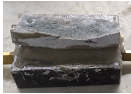
Figure D.62: Top debonded part of Specimen TG20-C-2
