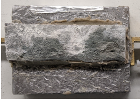
Figure D.47: Bottom debonded part of Specimen TG5-C-1
