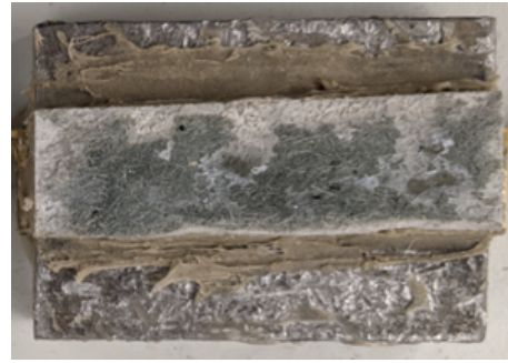
Figure D.36: Top debonded part of Specimen TG10-B-3
