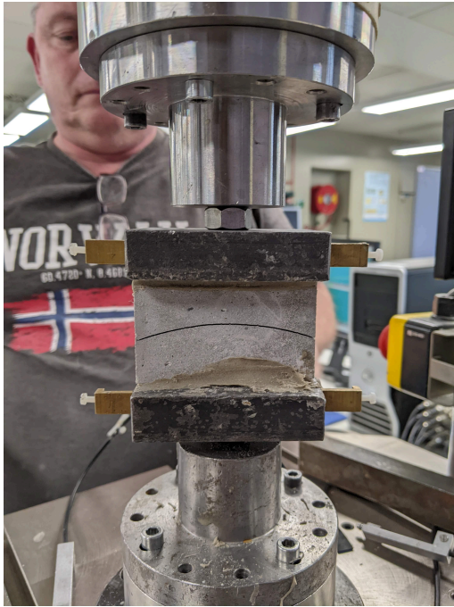
Figure C.41: Casted Specimen C-1 after failure
