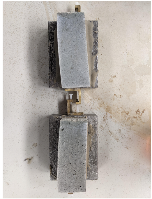
Figure D.76: Inter-layer surface of Casted Specimen C-3 after failure
