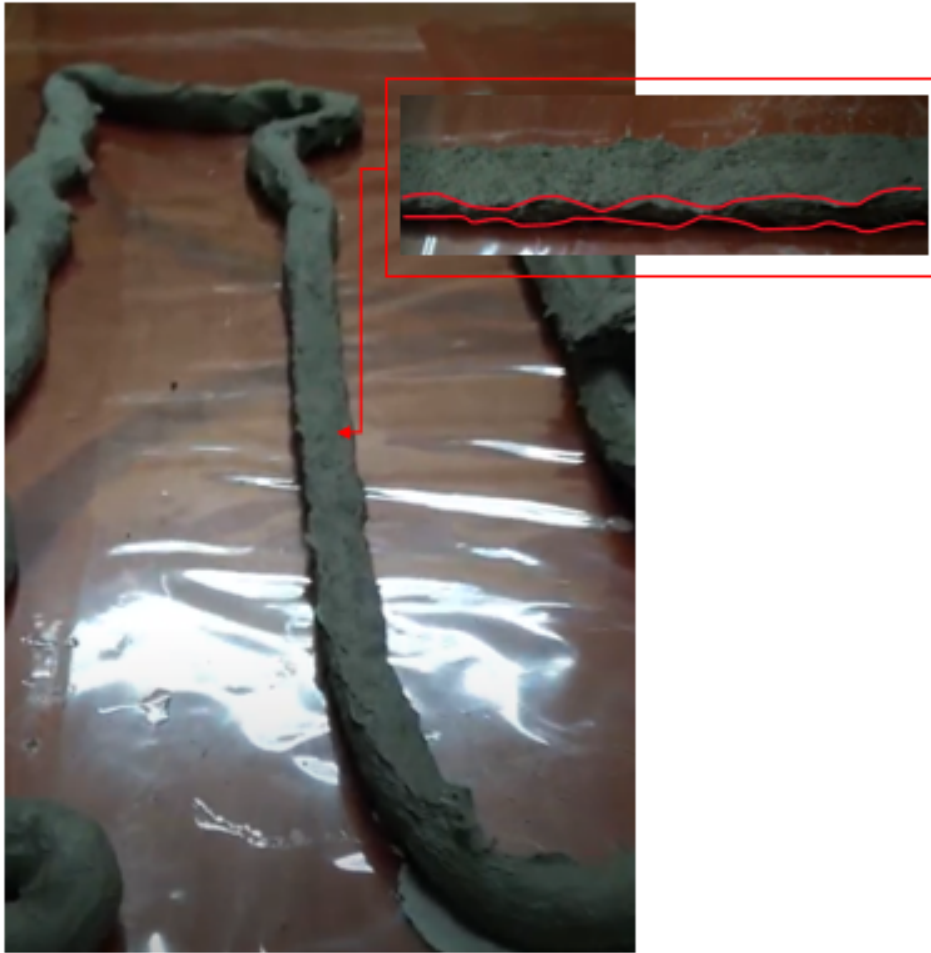
Figure A.7: Modified Nozzle Specimen printed by using extrusion-based 3D concrete printing (Zoomed in: Resulting osteomorphic block-based shape of extruded layer)
