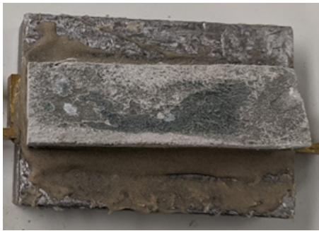
Figure D.65: Bottom debonded part of Specimen TG20-C-4
