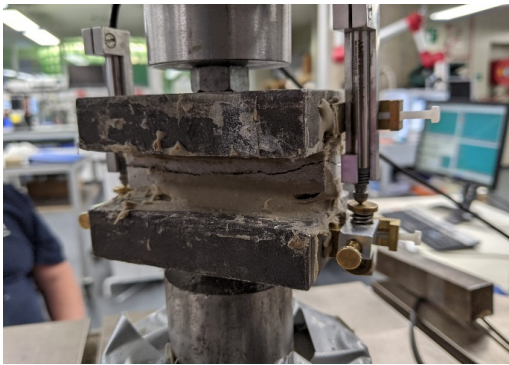
Figure C.18: Specimen TG10-B-3 after failure
