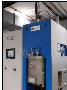
Figure 8: Spark Plasma Sintering machine
