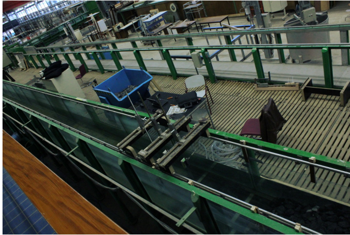
FIGURE F-1: OVERVIEW OF THE FLUME; WAVE GAUGES JUST IN FRONT OF THE SCALE MODEL
