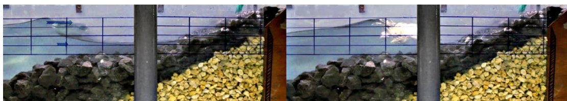
FIGURE 4.3-5: BREAKING WIND WAVES ON A PERMEABLE BERM BELOW SWL (BERM D)
