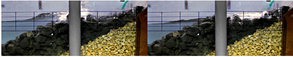
FIGURE 4.3-8: BREAKING WIND WAVES ON A PERMEABLE BERM ABOVE SWL (BERM F)
