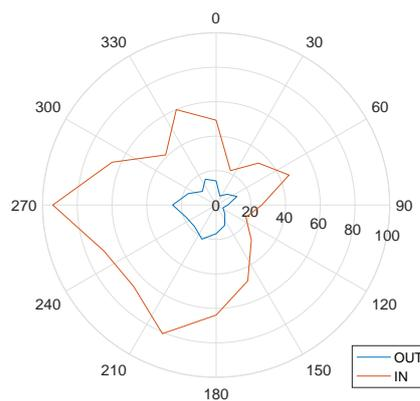
Figure 6.1: Energy rose showing in red the energy available in the local wind ( $E_{in}$ ) and in blue the energy produced by the wind turbine ( $E_{out}$ ). Radial axis in kilowatt-hour (kWh), time frame of one year.
