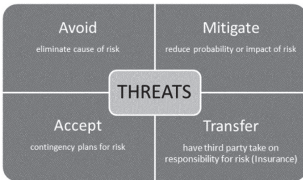
Figure 6: A mental model related to the fourth step of the basic cyber risk management cycle: risk response strategies (Dorfman 2007; Rowley 2014)
