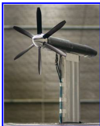
(a) Isolated propeller with six blades installed on a support pylon (propulsive regime).
