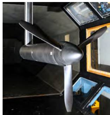
(b) Isolated propeller with three blades installed on a sting (regenerative regime).
