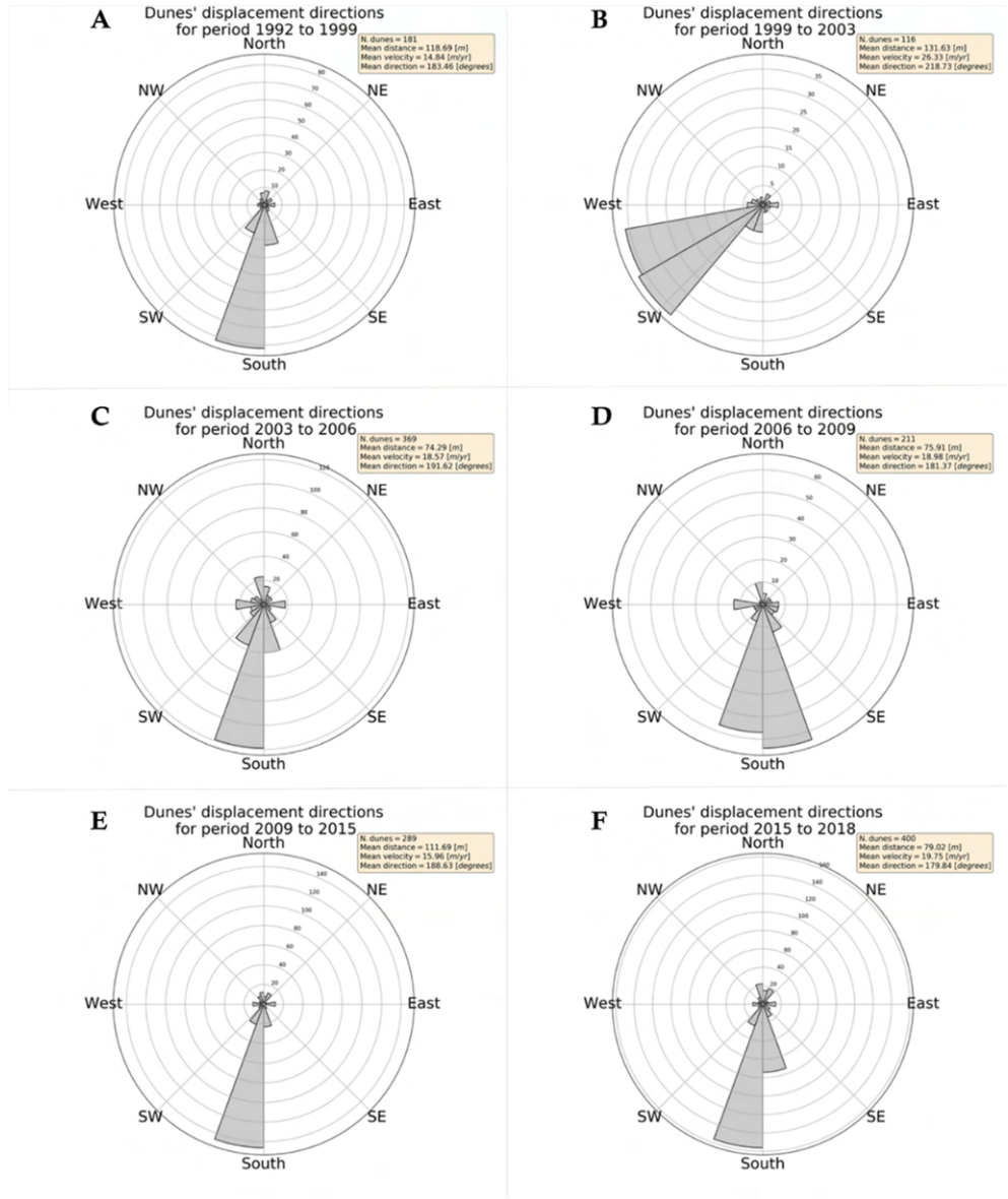
Figure 4.12: Dune displacement directions for the different periods analyzed, indicating the number of dunes and the mean values of migration distance, migration rate and direction or heading. A), C), E), F) show dunes displacement direction in SSW direction for the periods 1992-1999, 2003-2006, 2006-2009, 2009-2015 and 2015-2018 respectively. B) shows a dunes displacement direction in WSW for the intersensor period 1999-2003 and, D) shows a main displacement direction ranging from SSW-SSE for the period 2006-2009.
