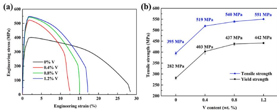
Fig. 3. Tensile properties of samples quenched at 1020 °C and tempered at 640 °C with different V content at 700 °C, (a) Stress-strain curves and (b) the variation of high-temperature strength.
