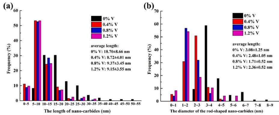
Fig. 6. The sizes of nano-carbides in samples quenched at 1020 °C and tempered at 640 °C with increasing V content, (a) the length, and (b) the cross-sectional diameter.
