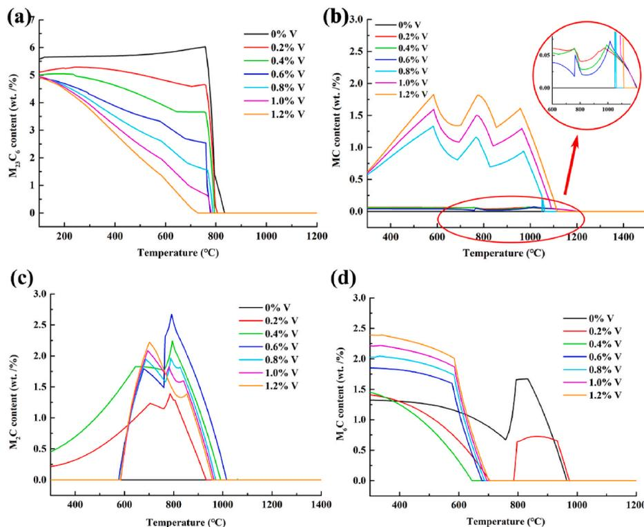
Fig. 1. Variations in carbide contents in the alloy with the increasing V content, (a)  $M_{23}C_6$ , (b) MC, (c)  $M_2C$  and (d)  $M_6C$  based on thermodynamic calculations of phase diagram.
