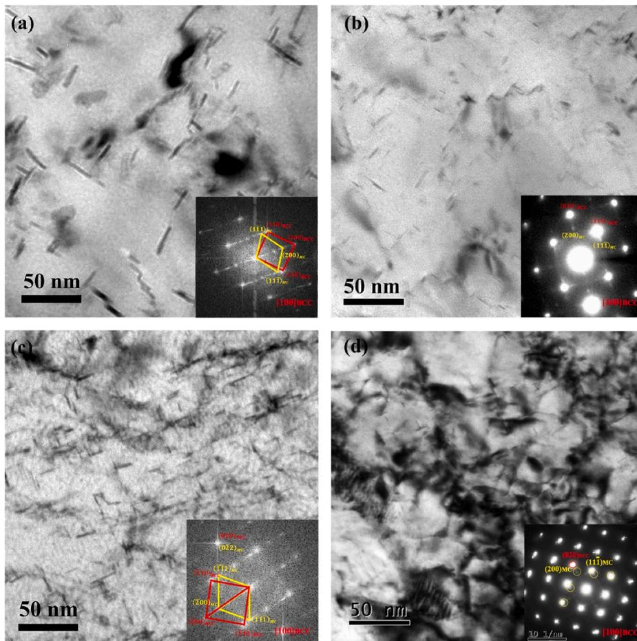
**Fig. 5.** The TEM micrographs containing nano-carbides in samples quenched at 1020 °C and tempered at 640 °C with different V contents of (a) 0% V, (b) 0.4% V, (c) 0.8% V, and (d) 1.2% V.
