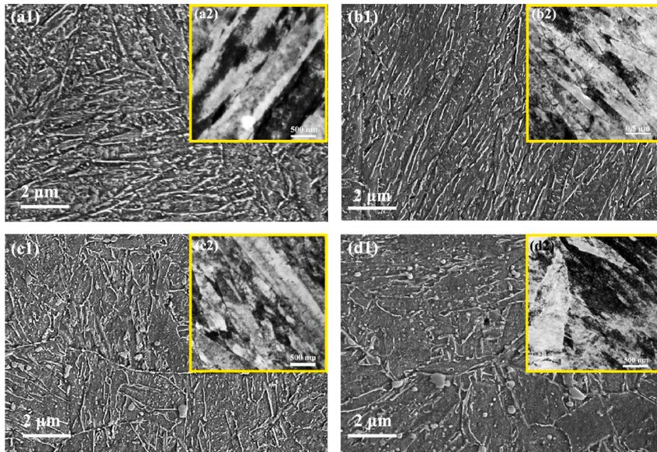
**Fig. 4.** The carbides and martensitic lath structure of samples quenched at 1020 °C and tempered at 640 °C, with different V contents of (a) 0% V, (b) 0.4% V, (c) 0.8% V, and (d) 1.2% V.
