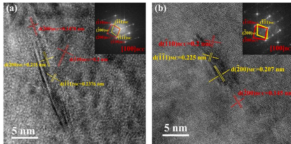
Fig. 7. HRTEM micrographs and the FFT pattern of nano-carbides in samples quenched at 1020 °C and tempered at 640 °C with different V contents of (a) 0% V sample, (b) 0.8% V sample.
