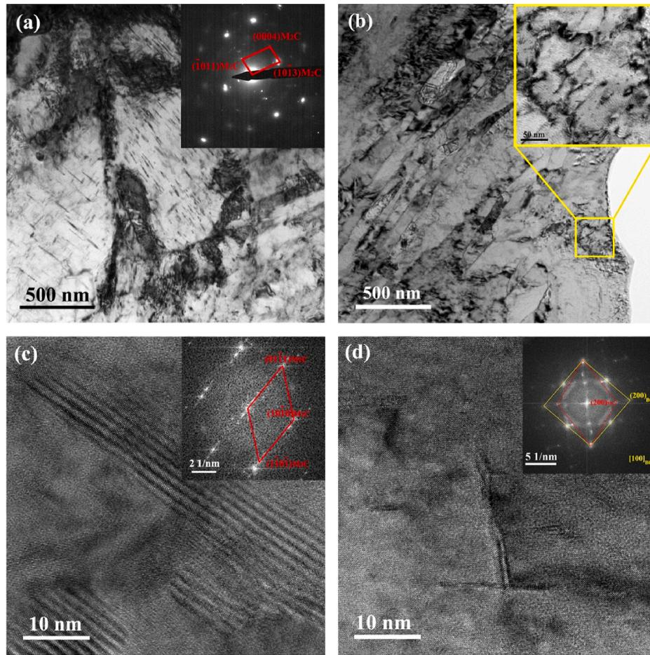
**Fig. 8.** Microstructure after high-temperature tensile test at 700 °C, TEM bright field images of (a) 0% V sample and (b) 0.8% V sample, and HRTEM micrographs of (c) M<sub>2</sub>C in 0% V sample and (d) MC in 0.8% V sample.
