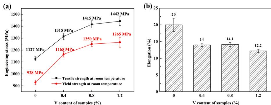
Fig. 2. Tensile properties of the samples quenched at 1020 °C and tempered at 640 °C, (a) tensile and yield strengths, and (b) elongation at room temperature.
