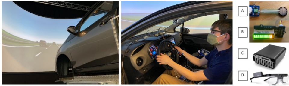
Figure 2.1: Experimental setup. Left side: Driving simulator (DAVSi) at Delft University of Technology. Middle: Participant with all measurement devices. Right side: (A) Pressure sensor for reporting continuous perceived risk. (B) LED bar- visual feedback of reported continuous perceived risk. (C) ECG device TMSi to measure cardiovascular activity. (D) Eye tracker Tobii pro 2 to measure pupil dilation
