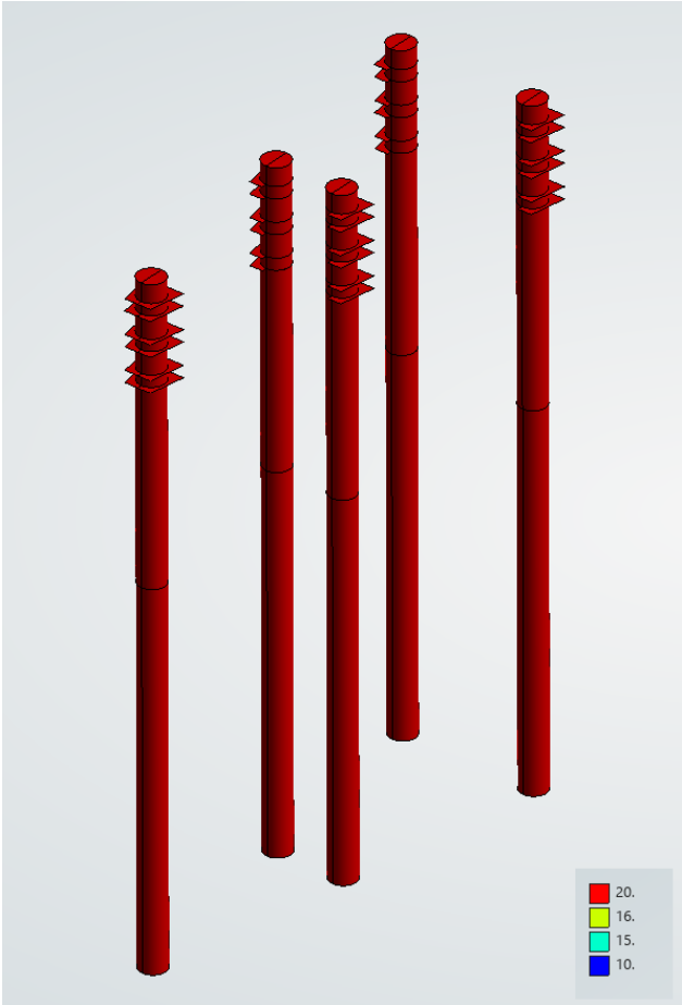
Figure B.13: Element thickness 20 mm: fender structure
