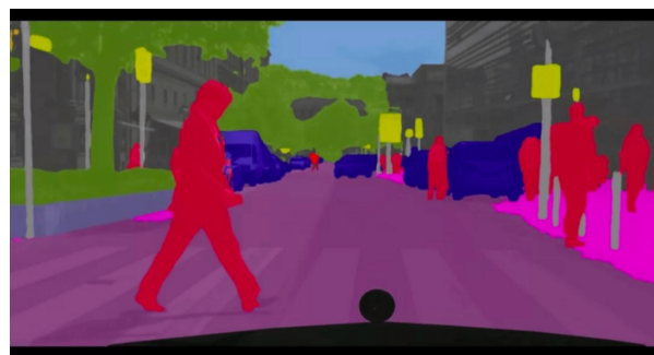
(b) Object Segmentation: each object's pixels are coloured uniquely for each class. [53]
