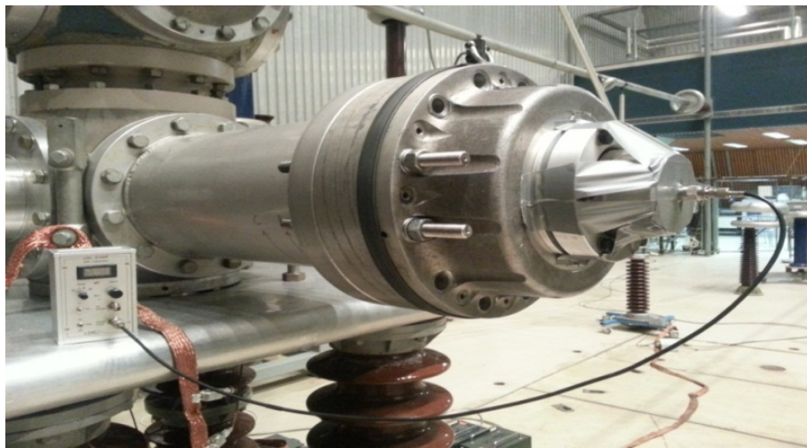
Figure D.1 – A pulse is injected through an external antenna mounted on the inspection window of the GIS.
