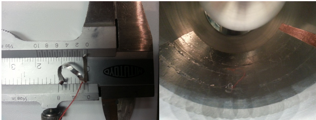
Figure 5.17 - The particle lays on the enclosure of the GIS. It is tied by means of the red cotton thread to the enclosure.
